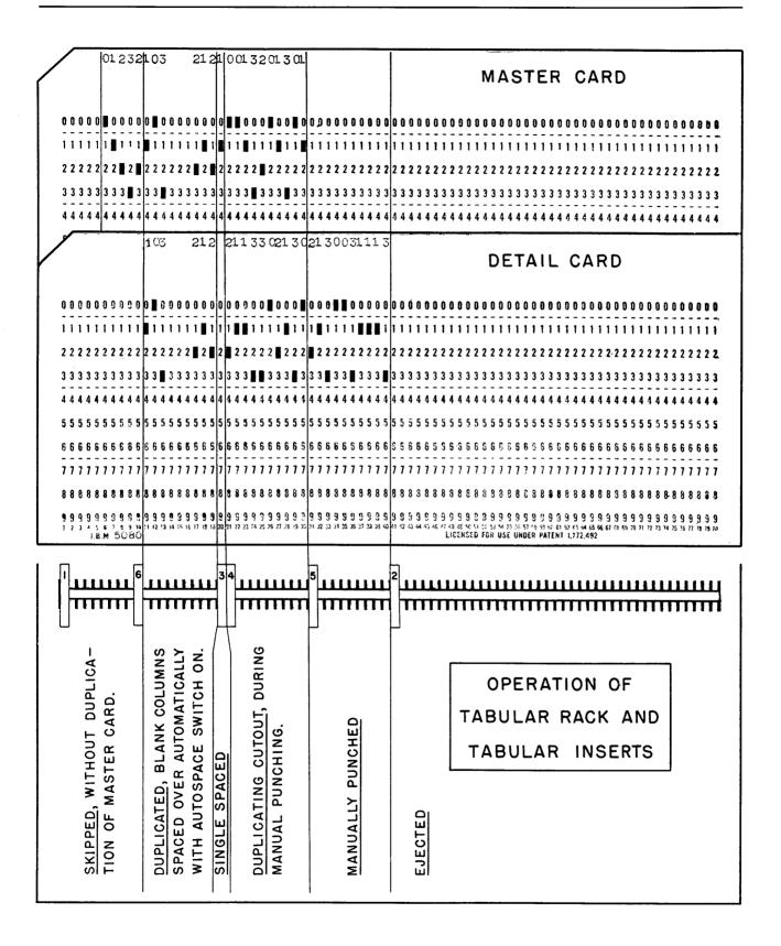
automatically by a tab start insert or manually by depression of the tab key. This stop insert must be placed in the last column position to be skipped, or, in other words, in the column position preceding that in which punching is to be resumed.
