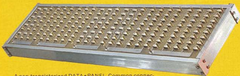
A non-transistorized DATA•PANEL. Common connection for one side of lamp supply simplifies hook up. Taper pin receptacle used for signal connection. Lamps are replaced by moving center contact aside.
