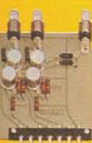
Printed circuit cards contain complete lamp control circuitry. Size varies with indication requirements.
