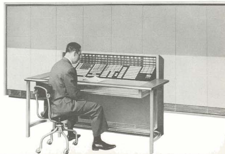
Computer —Automatic program control over up to 63 magnetic tape stations, up to 12 random access files.
