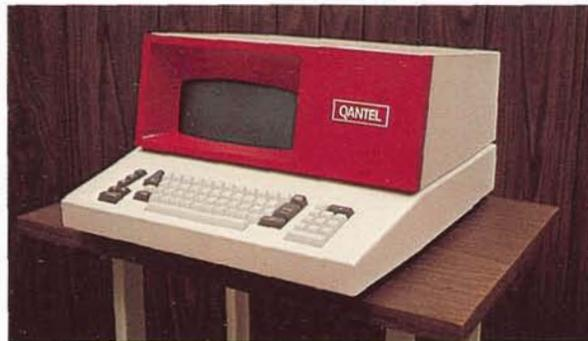
QANTEL Model 4001 Video Terminal features a 960-character screen, extra large characters (upper and lower case), automatic right-justification of numeric entries and a familiar typewriter keyboard, plus a numeric-key cluster. Automatic polling and response capabilities are standard.
