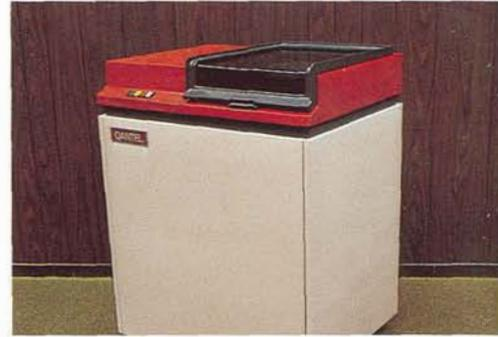
QANTEL Model 3201 Disc Drive provides 30 million characters of quickly accessible data storage. Four Model 3201 Disc Drives can be supported by Systems 1100 and 1200, giving up to 120 million characters of disc storage.
