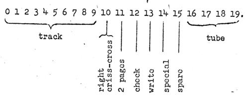
A special magnetic instruction (input-output) is interpreted according to its 3rd character as follows
