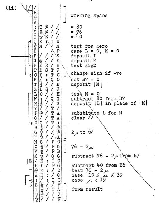
Note: Lines: / and S/ are used as working space so that as it stands the sequence of instructions is not self-resetting, i.e., it cannot be used again unless the instructions in these lines are restored.
