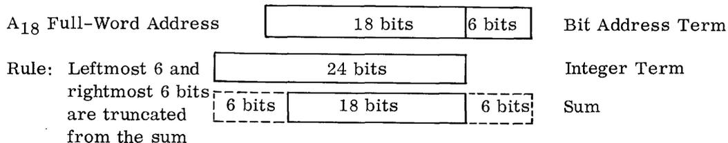
Note: An integer in an 18-bit field counts full words or unit address, control operation, control word address, and so on, in right I-O address.
