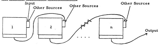
In this way a chaining process can be set up whereby memory 1 is making the 1st lookup on the  $p^{th}$  sequence of lookups, memory 2 is making the 2nd lookup on the  $(p - 1)^{th}$  sequence, and memory n is making the last  $(n^{th})$  lookup on the  $(p - n)^{th}$  sequence. The result of this approach is that if there are n memories and n lookups to a sequence the total time for the sequence of lookups averages approximately 1 memory reference time.
