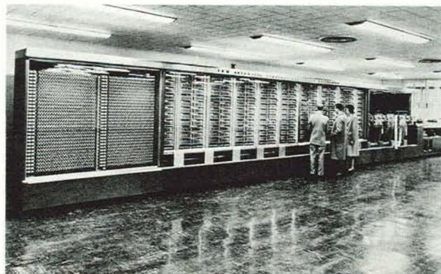
In 1944, Harvard's Dr. Howard Aiken and IBM completed five years of work on the Mark I, the largest electromechanical calculator ever built. It had 3,300 relays and weighed 5 tons. It could multiply two 23-digit numbers in six seconds.
