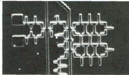
How dense is dense? When magnetic disks were first introduced, it was possible to pack 1,000 bits of data per square inch. Today the number is several million. But another technology called magnetic bubbles—still in the research stage—may increase density even further. Bubbles are tiny magnetic regions found in certain thin magnetic materials.
