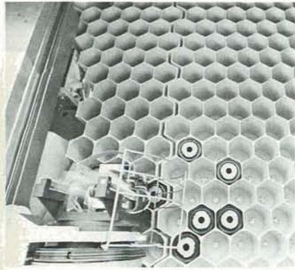
← The IBM 3850 Mass Storage System—a beehive of electronic activity. It contains up to 472 billion characters of information. Cartridges in each honeycomb cell contain magnetic tape. On signal, data on tape is transferred to disks, then to computer memory. Introduced in 1975, the 3850 gives quick and inexpensive access to vast files of data.
