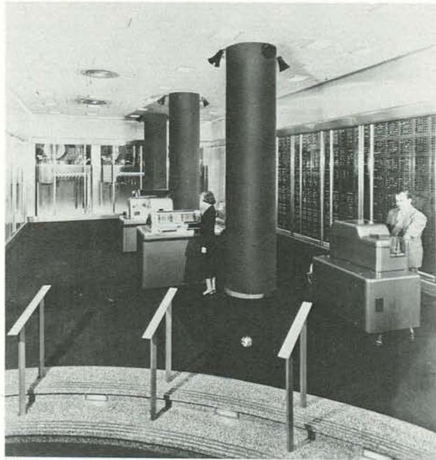
↑ The IBM Selective Sequence Electronic Calculator, completed in 1947, contained both vacuum tubes and relays. It was more than 100 times faster than the Mark I. It was the first IBM stored program machine, and it could select its own calculating sequence by modifying its own stored instructions—thus, its name.
