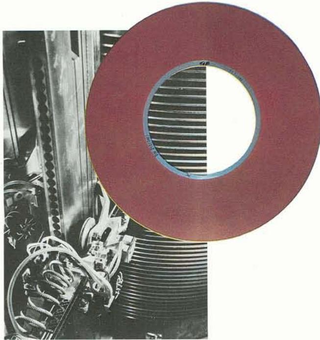
← When IBM introduced its 305 RAMAC (for random access) in 1956, data processing leapfrogged into the future. Magnetically coated aluminum disks (such as miniature replica at left) stored volumes of data on concentric tracks. In a fraction of a second, a read/write mechanism found the right magnetic spot and retrieved data from any point on the disk. The RAMAC's 50 spinning disks contained five million characters of information.
