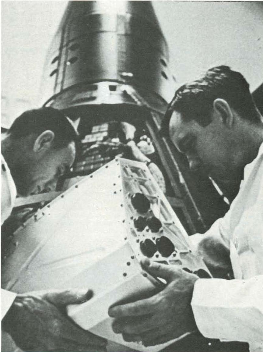
↑ Small and rugged, this onboard 59-pound computer helped guide Gemini spaceflights through rendezvous, docking, and splashdown. For guidance and navigation, IBM developed another family of computers, called 4 Pi. In many applications, magnetic drums were used for storage because of durability, size, and quicker access time.
