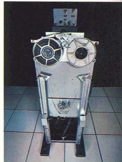
↑ The vacuum tape column, invented by IBM in 1950, controlled the reeling and unreeling of tape and kept it from snapping. Vacuum columns are at left and right, under reels.
