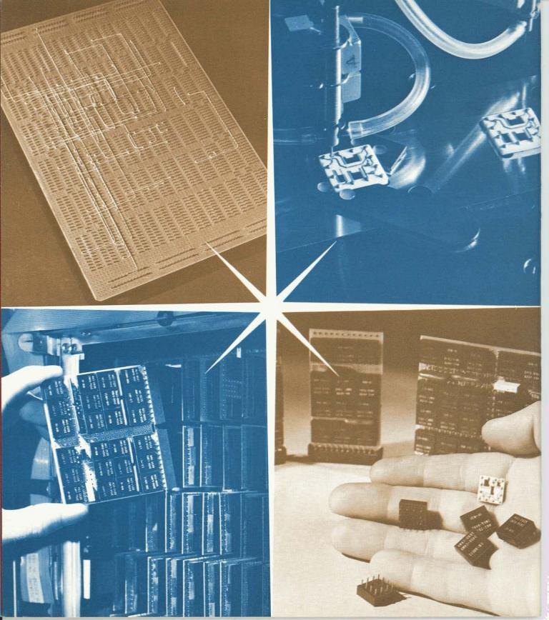
leave a logic card via contacts that connect to pins on a circuit board. Each logic card provides printed conductors for distributing voltages and signals between module circuit points and card pins.
