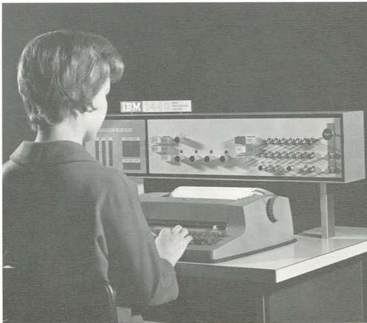
When application coverage or processing conditions require more program flexibility and faster program execution, special features can be added to a 1440 Data Processing System.
