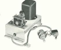
The repetitive oscillator allows problem solutions to be displayed on an oscilloscope.
