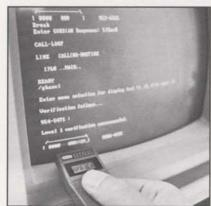
Charlie Dickman demonstrates the use of the Gordian Key Access device, which can be held in the palm of the hand, and with a numerical keypad can be adapted for screens that do not allow direct interaction.
