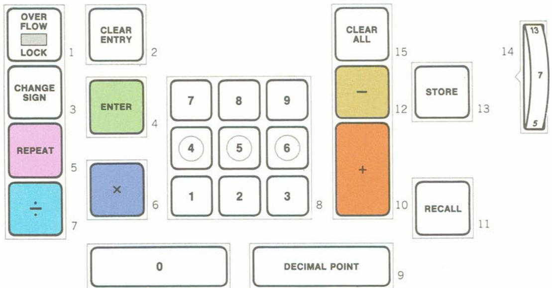
This is the simple "11-key" keyboard of the Friden Electronic Calculator. Everything is grouped in a convenient pattern within the span of the human hand. All controls are clearly marked and easy to use. The Decimal Point key allows you to enter amounts just as you would write them. The Store key lets you retain constant factors or results in a memory unit, while the Recall key lets you bring them back at any time for further calculation.
