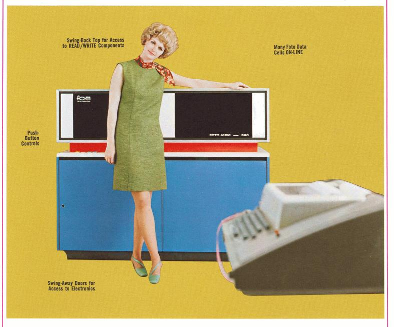
Operation of the FM 390 is extremely simple. The associated computer controls the functions of the System. Internally, a maintenance Control Panel enables operation of the other functions previously listed under System Components. The FM 390 is designed for easy access to the electronics in the bottom section by means of doors. The top of the unit swings back to enable access to both READ and WRITE components.
