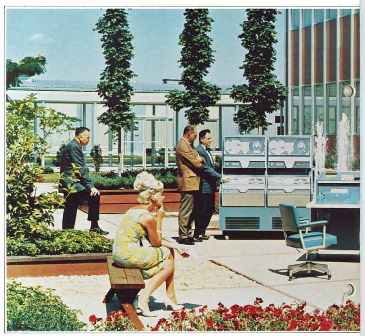
ties of 556 and 800 bits-per-inch on half inch 9-track magnetic tape. One controller can handle up to four tape transports and provides word assembly/disassembly. Magnetic Tape System (includes one transport expandable to 4.) Additional Magnetic Tape Transport 640/730.
