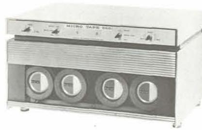
tracks in the Phase Recording System at densities of 375 bits per track inch and may be transferred at a rate of 90,000 bits per second. Tape handling and utility transfer routines available.
