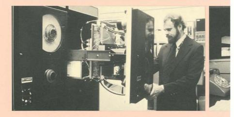
The RS03's capacity is 512K bytes; the RS04's is 1024K bytes. Both drives can be mixed on the same controller and are software compatible.
