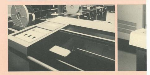
The LP11 Line Printers – The LP11 line printer series starts with a 132-column, 64-character model, the LP11-V, which operates at 300 lines per minute. The LP11-W version, which uses a 96character set, runs at 230 lines per minute.
