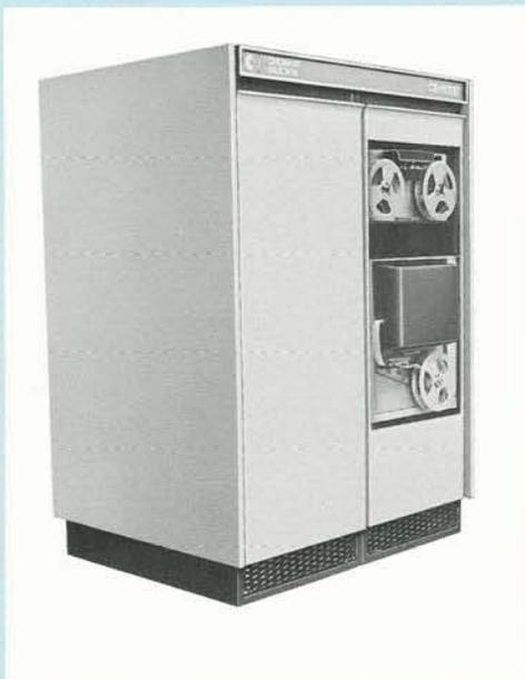
The auxiliary cabinet of the CIP/4000 which contains the I/O module, the tape reader, and the DRPE punch.
