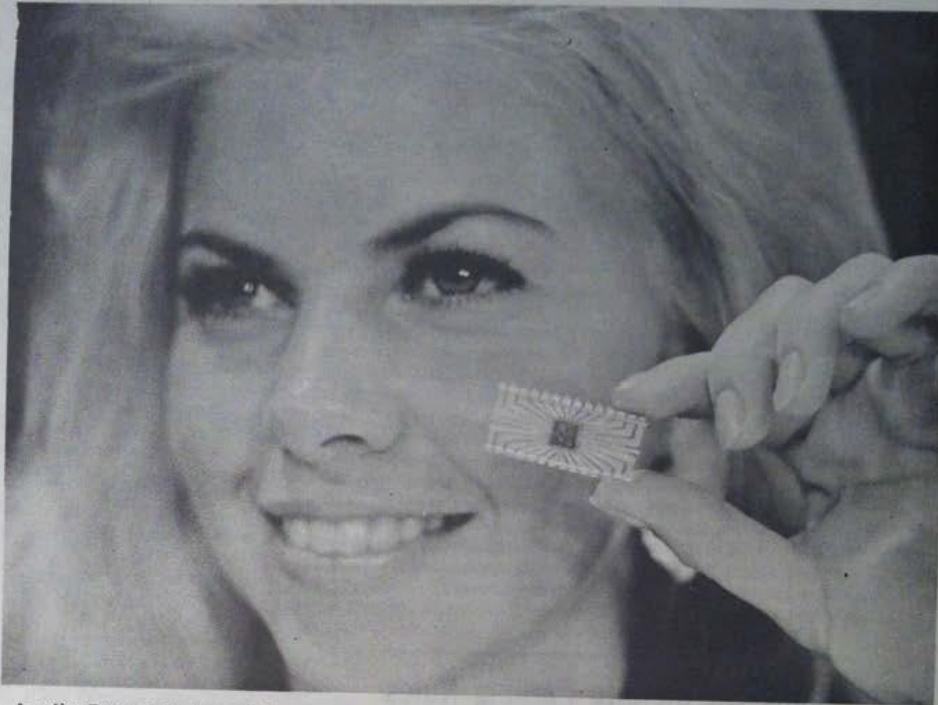
Amelia Rust of Equipment Group, Dallas, displays the "Calculator on a Chip", a complex integrated circuit containing all the logic and memory functions necessary for an eight-digit calculator. The device was named "Circuit of the Year" by a German electronics publication.
