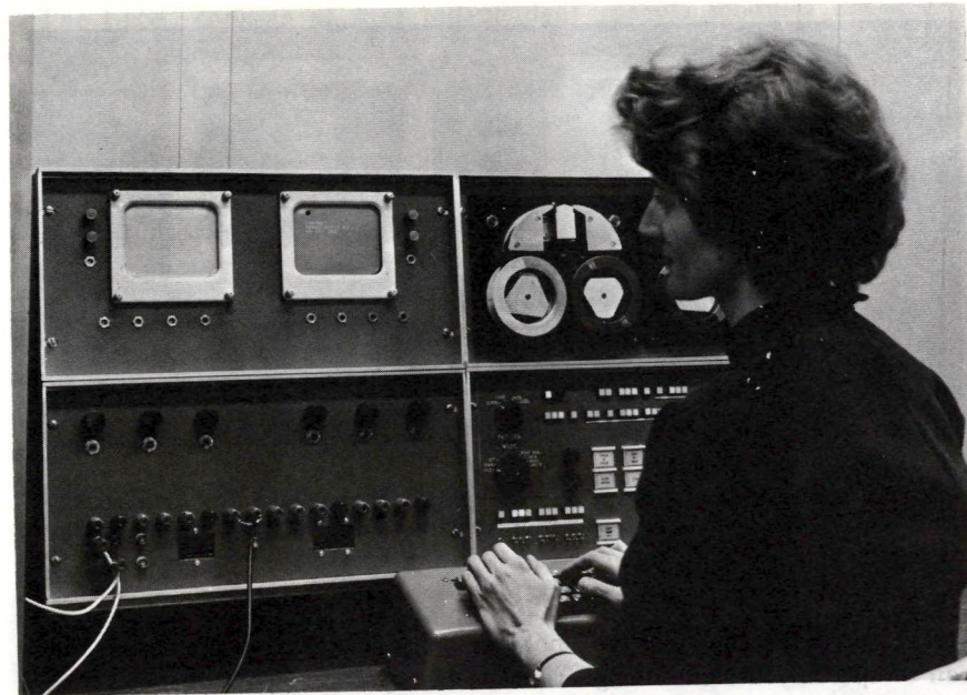
FIGURE 4. Information typed on the keyboard and displayed on the scope is simultaneously stored in the central memory. From here it may be transferred to magnetic tape and recovered whenever desired.
