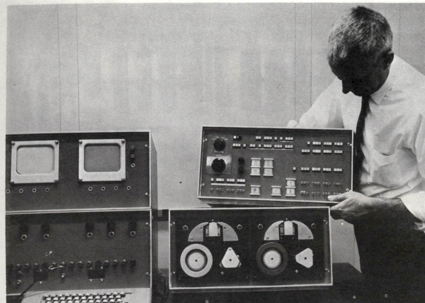
FIGURE 10. The control module being stacked on top of the magnetic tape module. Cables connecting console panels to the electronics cabinet are plugged in from the rear.
