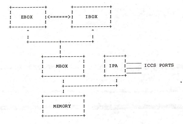
The internal CPU structure looks very similar to the DOLPHIN. There is a IBOX and an EBOX to allow two instructions to get executed at once and an MBOX with a 4K cache. However, the DOLPHIN bus has been eliminated. This provides the following advantages:
