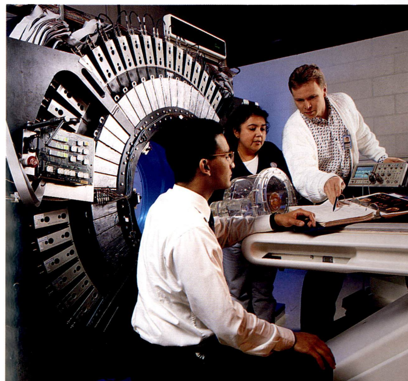
Michael Britton, Maria Trinidad and Peter Crandall (left to right) are members of a co-located GE Medical Systems team that developed a new generation of Positron Emission Tomography (PET) scanner. Introduced by GE in 1992, the Advance™ imager above is designed for image quality, patient throughput and ease of use. Physicians use PET images to evaluate a variety of diseases, including cancer and epilepsy.
