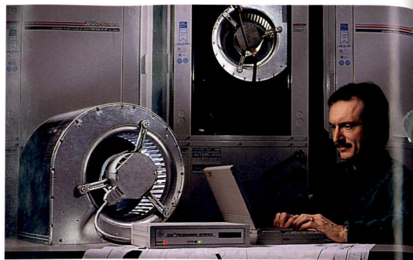
Brian Beifus of GE programs the memory chip inside a new ECM™ motor for use in a geothermal heat pump unit made by WaterFurnace.
