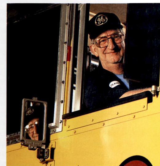
Clarence Garver, an employee in the locomotive business, found a simple solution to a customer problem, thereby avoiding a costly redesign. His idea, called a "switching step observation system," was to use a small forward-facing mirror in conjunction with the standard side-view mirror to give locomotive operators a clear view of the front of the locomotive. A patent is pending for the idea.
