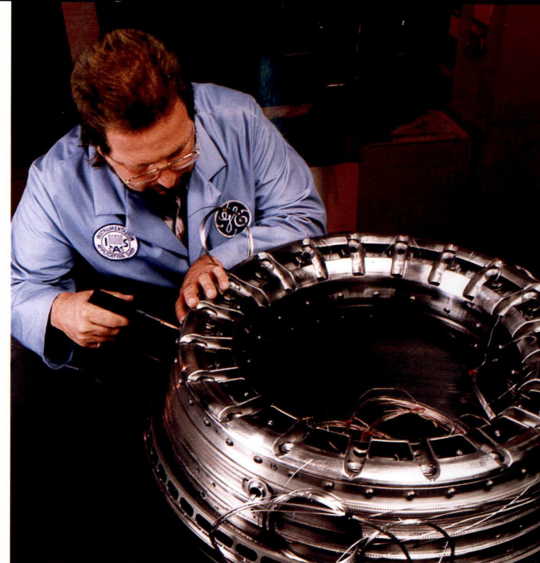
GE Aircraft Engines has developed a low-emission, dual-annular combustor, a key element in what soon will be the cleanest burning jet engines. Based on technology from NASA's Energy Efficient Engine program, the new combustor design has been incorporated into the super-high-thrust GE90, which will enter service with British Airways in 1995, and into the CFM56-5B, which will enter service with Swissair and Austrian Airlines the same year. Here, Roger DeBruler of GE prepares a combustor for component testing.
