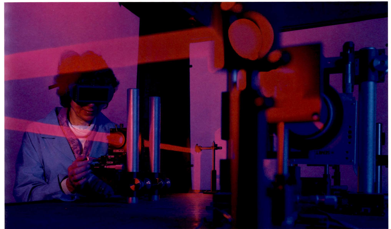
RESEARCH MANAGER KATHRYN CHALFAN DEMONSTRATES OPERATION OF THE FIRST OPTICAL ADAPTIVE RESONANCE NEURAL NETWORK. BOEING EXPERIMENTS WITH THIS DEVICE COULD LEAD TO SPECIAL-PURPOSE OPTICAL SUPERCOMPUTERS.
