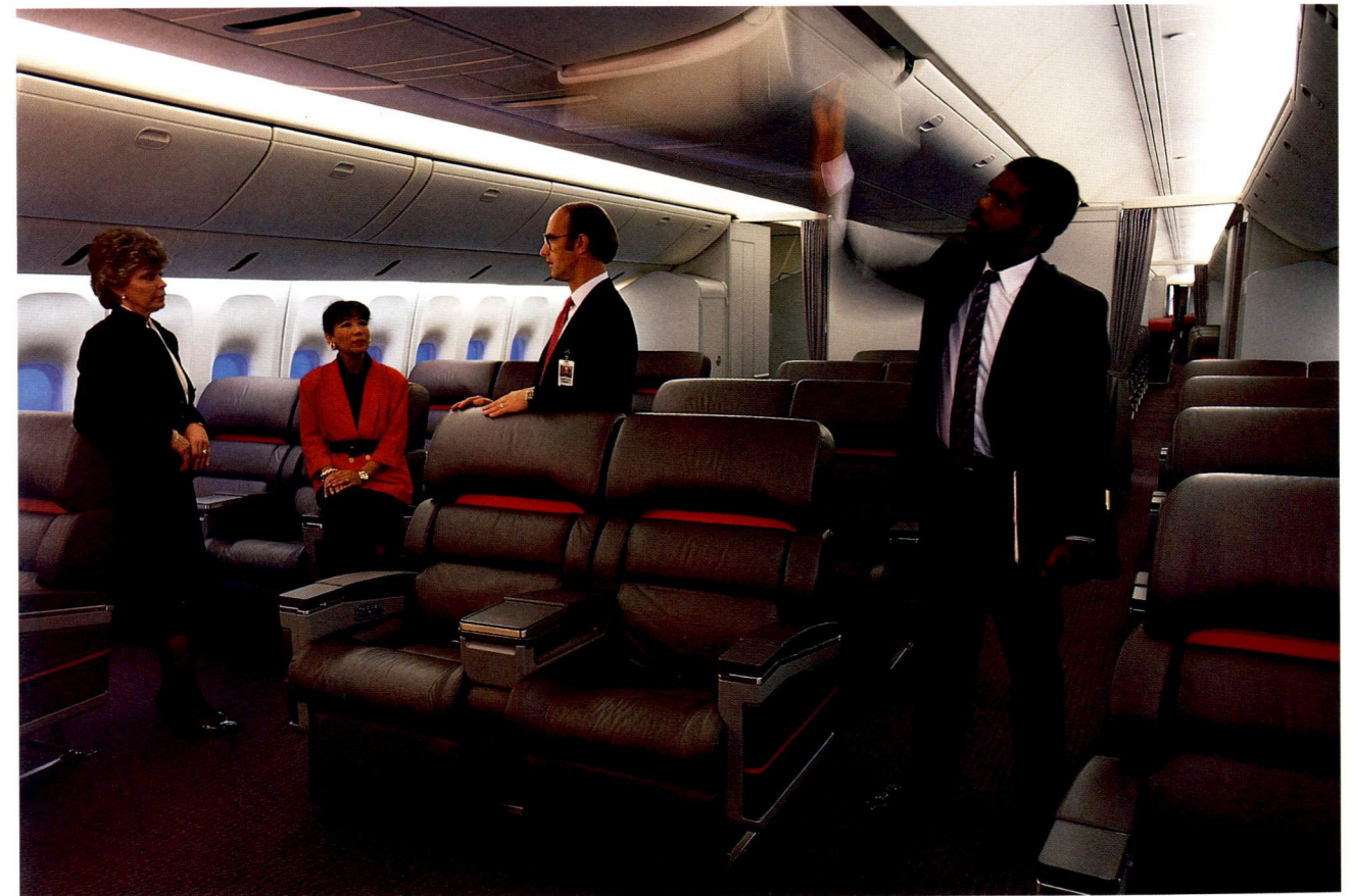
FULL-SCALE MOCK-UP OF 777 INTERIOR CABIN IS USED TO ACQUAINT AIRLINE REPRESENTATIVES AND PROGRAM PERSONNEL WITH THE AIRCRAFT'S MANY ADVANCED FEATURES, SUCH AS LARGER OVERHEAD STORAGE BINS, EXTRA HEADROOM, AND FLEXIBLE SEATING OPTIONS.
