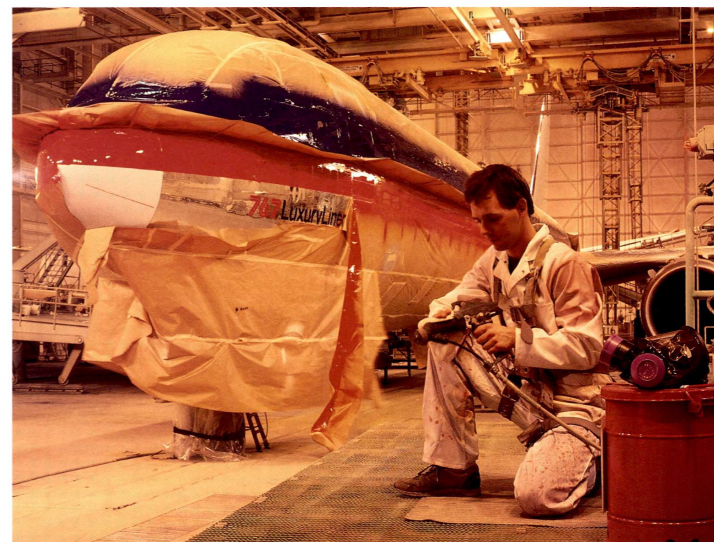
SAFETY AND ENVIRONMENTAL PROTECTION ARE TOP PRIORITIES AT ALL BOEING FACILITIES. HERE, AT THE COMPANY'S EVERETT, WASH., PLANT, PAINTER CLINT HUSEBY READIES A SPECIAL SPRAY GUN THAT ELECTROSTATICALLY CHARGES THE PAINT SO THAT IT IS DRAWN TO THE AIRPLANE — RESULTING IN FEWER PAINT PARTICLES IN THE AIR.
