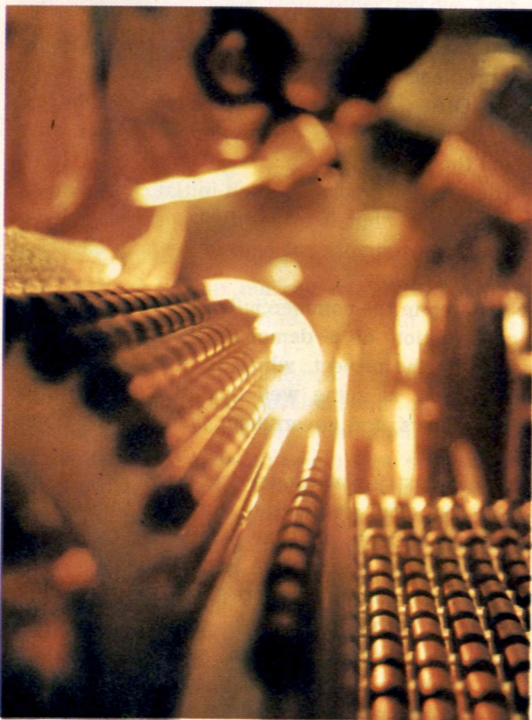
Tiny pellets of uranium dioxide, the fuel of a nuclear reactor, are manufactured under meticulous quality control conditions.
