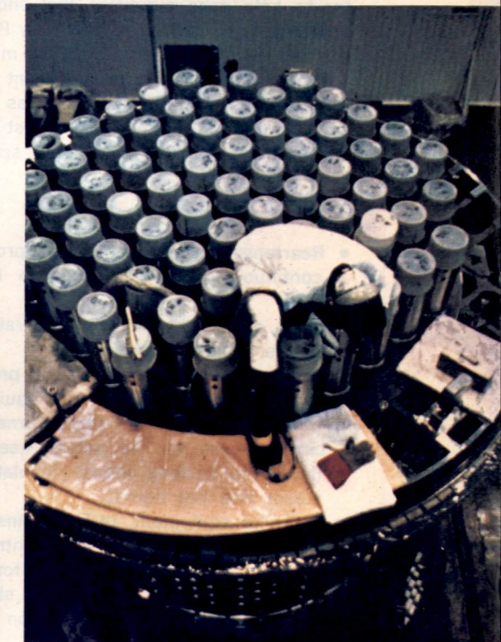
An 800-ton nuclear vessel leaves a Babcock & Wilcox Co. Mount Vernon, Ind., plant. When installed, heat from the nuclear reaction contained in the vessel will produce steam sufficient to generate 800,000 kw of electrical power. In another operation, nuclear fuel control rod guide assemblies are test assembled (below) in a reactor vessel simulator stand prior to shipment.
