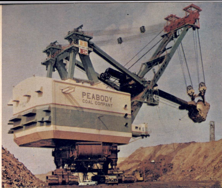
Huge Bucyrus-Erie shovel dwarfs more conventional vehicles as it harvests coal in Illinois. The bucket has a capacity of 140 cu yd.
