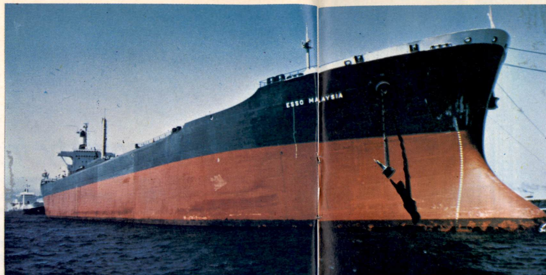
One of the new breed of supertankers, the Esso Malaysia is rated at 190,000 dead weight tons and has been in service since 1968. Newer and larger tankers already in service are rated as large as 321,000 dwt.
