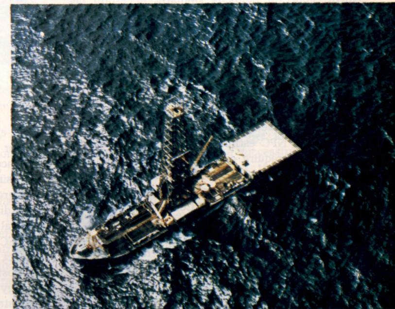
One of the new breed of supertankers, the Esso Malaysia is rated at 190,000 dead weight tons and has been in service since 1968. Newer and larger tankers already in service are rated as large as 321,000 dwt.
