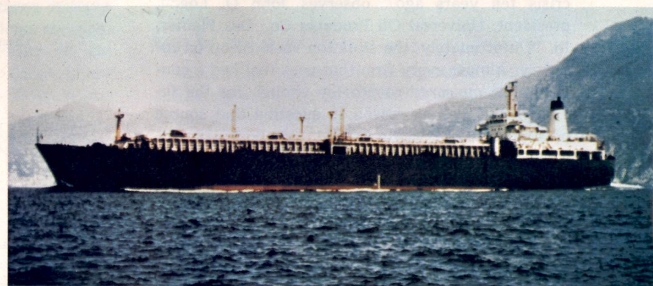
Recent addition to the high seas is the "floating Thermos bottle"—the tanker designed to transport liquefied natural gas (LNG). The Esso Brega carries 250,000 barrels of LNG in four insulated aluminum tanks at a temperature of -260 F.
