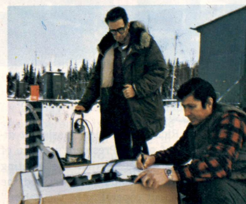
Two technicians take moisture and density readings with a nuclear probe at the Fairbanks test facility of the University of Alaska. The tests are to determine the possible effect of the transalaskan pipeline system on the environment.
