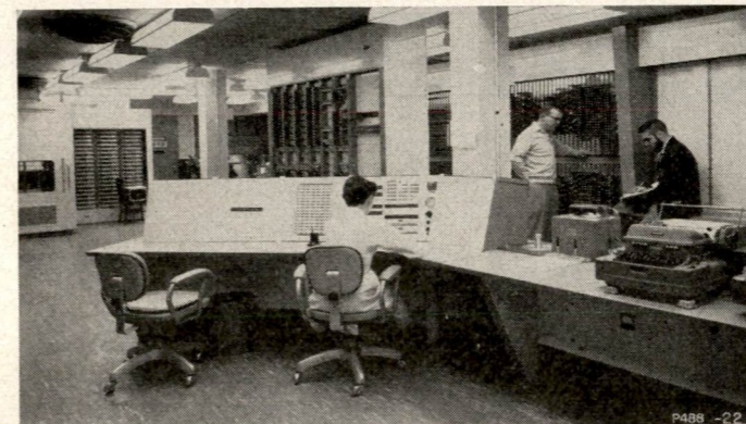
Fig. 1—The Lincoln TX-0 and TX-2 computers. Foreground: TX-0 console; middle center: TX-0 central computer frame; right rear: partially completed TX-2 frame showing plug-in unit construction; left rear: the 256×256 memory.
