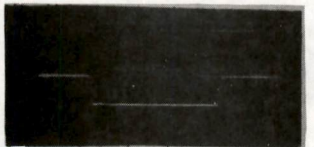
FIG. 12 1.8\mu\text{ SEC} CORE DRIVER OUTPUT PULSE
