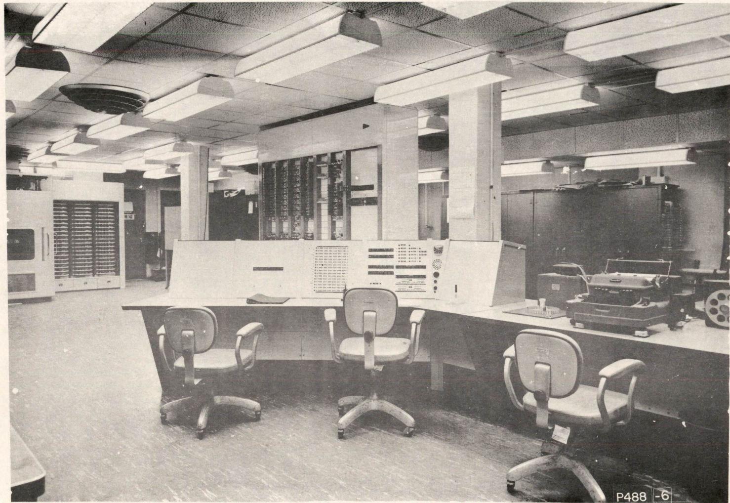
FIG. 1 TX-O COMPUTER ROOM
