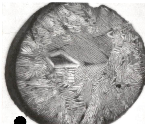
This is a chunk of sea water frozen in the lab. At 3x magnification the tiny platelets stand out clearly.
