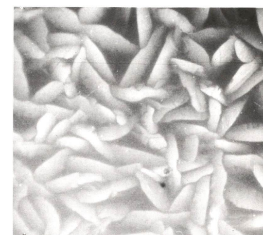
... In ice frozen slowly, the plates are more spread out. The goal: Fast freezing with plates still separated.
