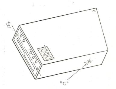
B) LOCK SCREW "C" IS PUT INTO CORRECT LOCATION, CENTERED AS SHOWN AND TIGHTENED.
