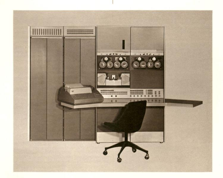
without waiting for the memory to store the word. Similarly, when reading a word out of memory, the processor takes the information and operates on it immediately, without waiting for the memory to finish the rewrite portion of its cycle.
