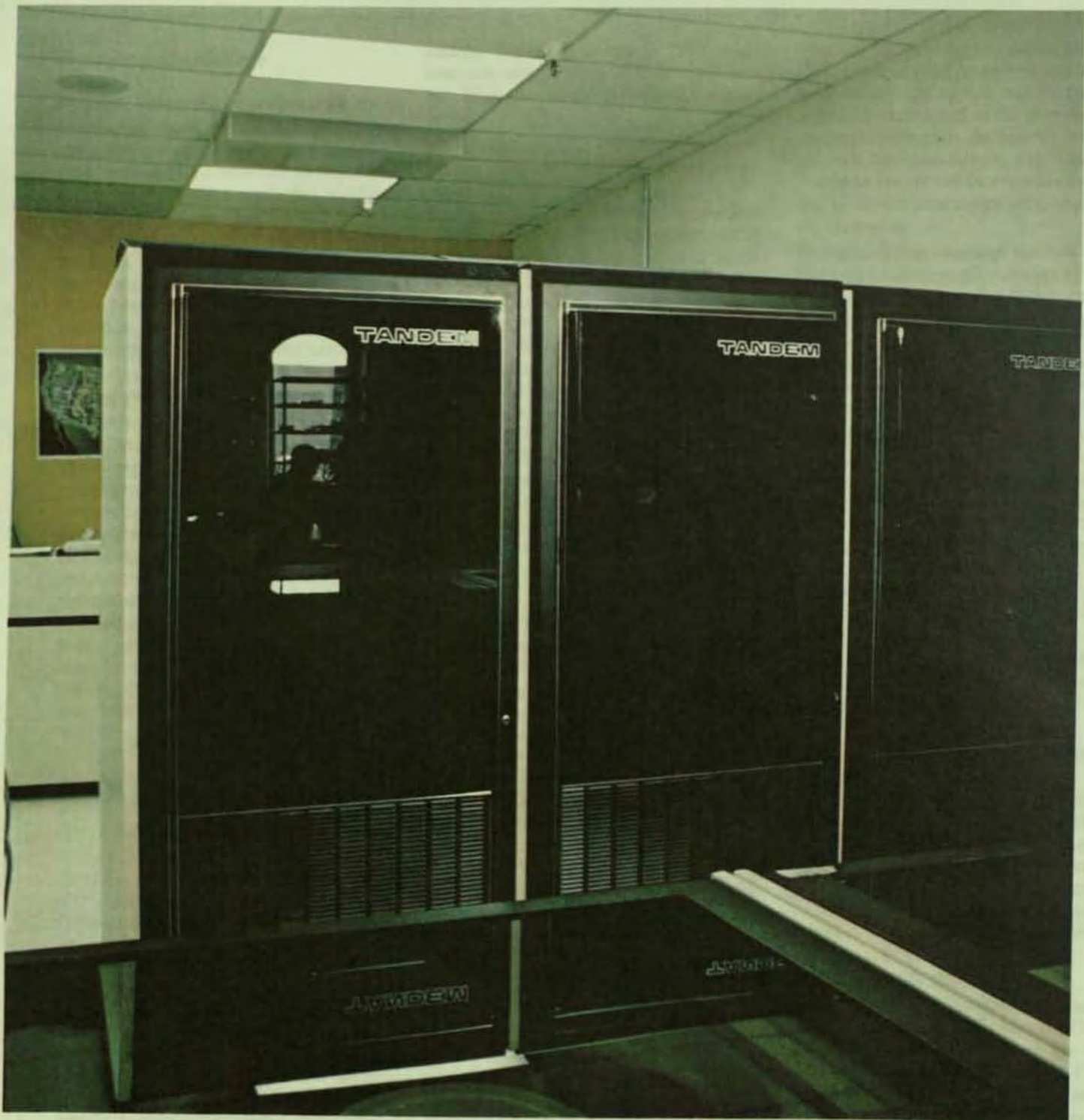
Tandem four processor system, expandable to six in same cabinetry, expandable to sixteen processors with additional cabinetry.
