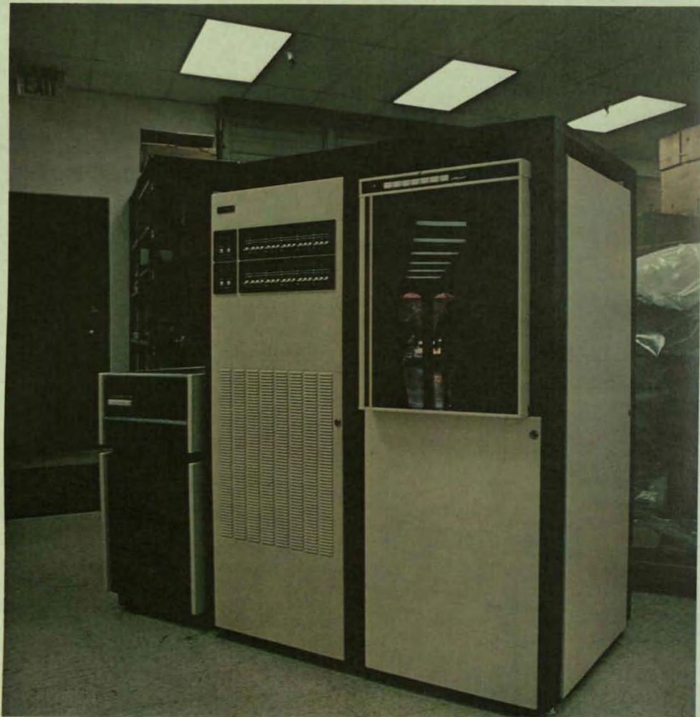
Dual processor system cabinet utilizing standard 19" rack mountable modules.
