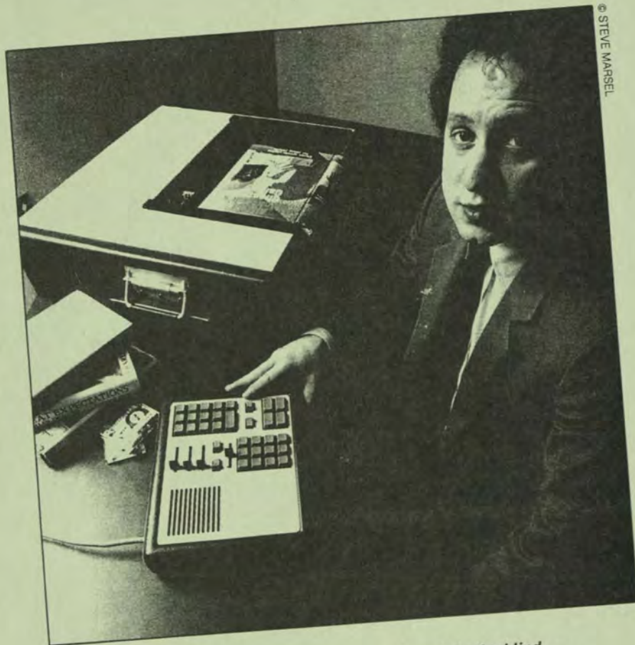
Ray Kurzweil's Reading Machine scans texts and reads to the blind.
