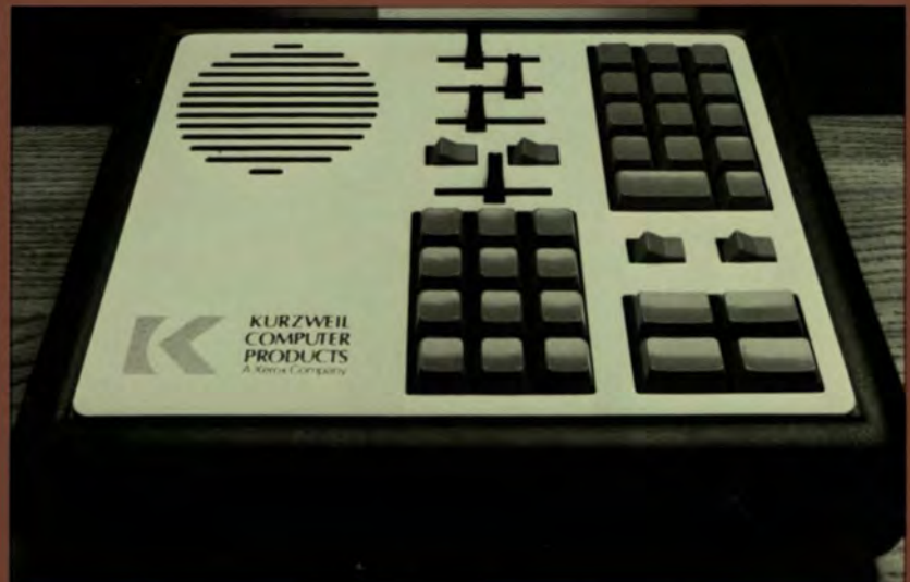
The control panel provides extensive tools for text and speech manipulation, with an audible description of each key if needed. The panel also doubles as a scientific calculator.
