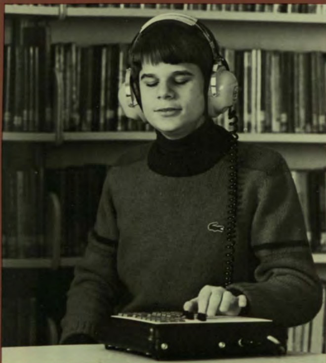
Children quickly master the KRM's controls. A headphone option permits them to use the system without disturbing others.
