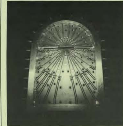
The primary advantages of BAW technology are its simple architecture (it's a monolithic structure), its small size (it's smaller than a golf ball), its passive nature (no operating power is required), and its low production costs (they are built efficiently, like integrated circuits). Add to that, its extraordinary capabilities, and it's easy to see there's a big place for BAW technology in ATD's future.
