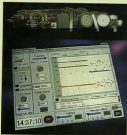
Advent Systems' portable polarimeter rapidly measures RF signal polarization parameters.
