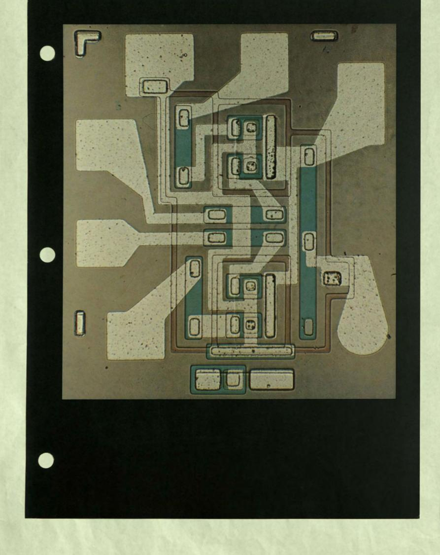
The backbone of Fairchild's diode-transistor logic (DTL) family, this master-slave flip-flop was the first static flip-flop in the semiconductor industry.
