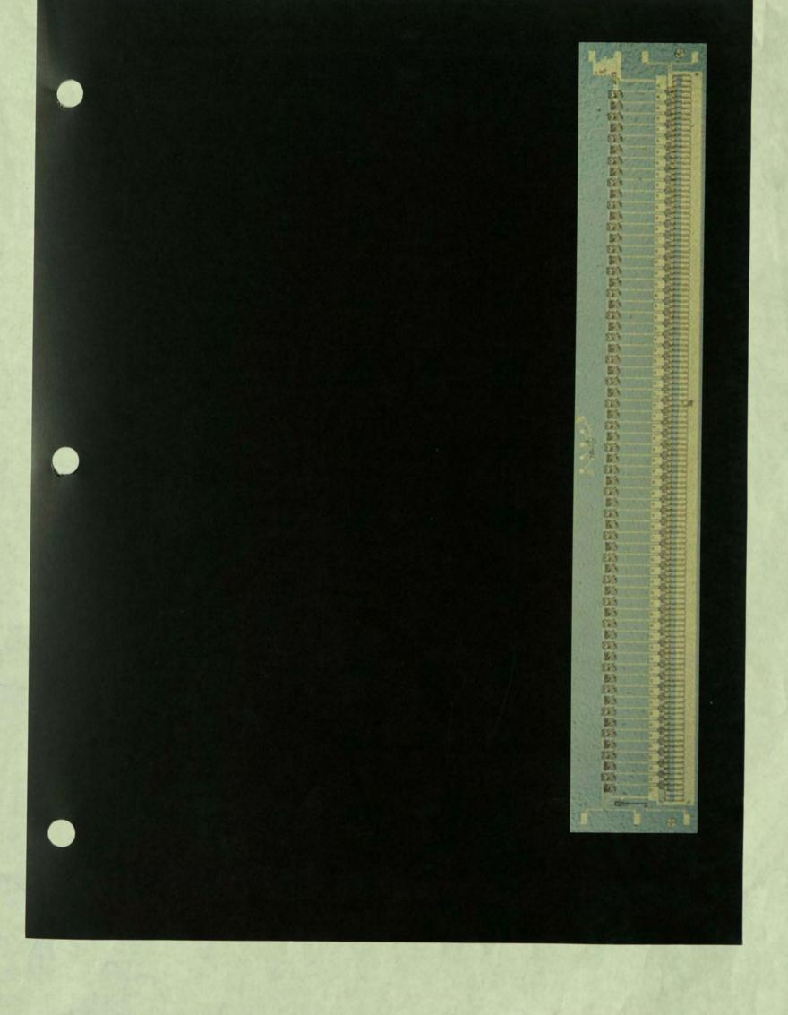
This silicon-gate MOS Micromosaic circuit shows the impact of custom technology on the semiconductor environment. Developed for Philips of France, the complex 400-gate design provides the digital logic portion of a duplex data communications system.
