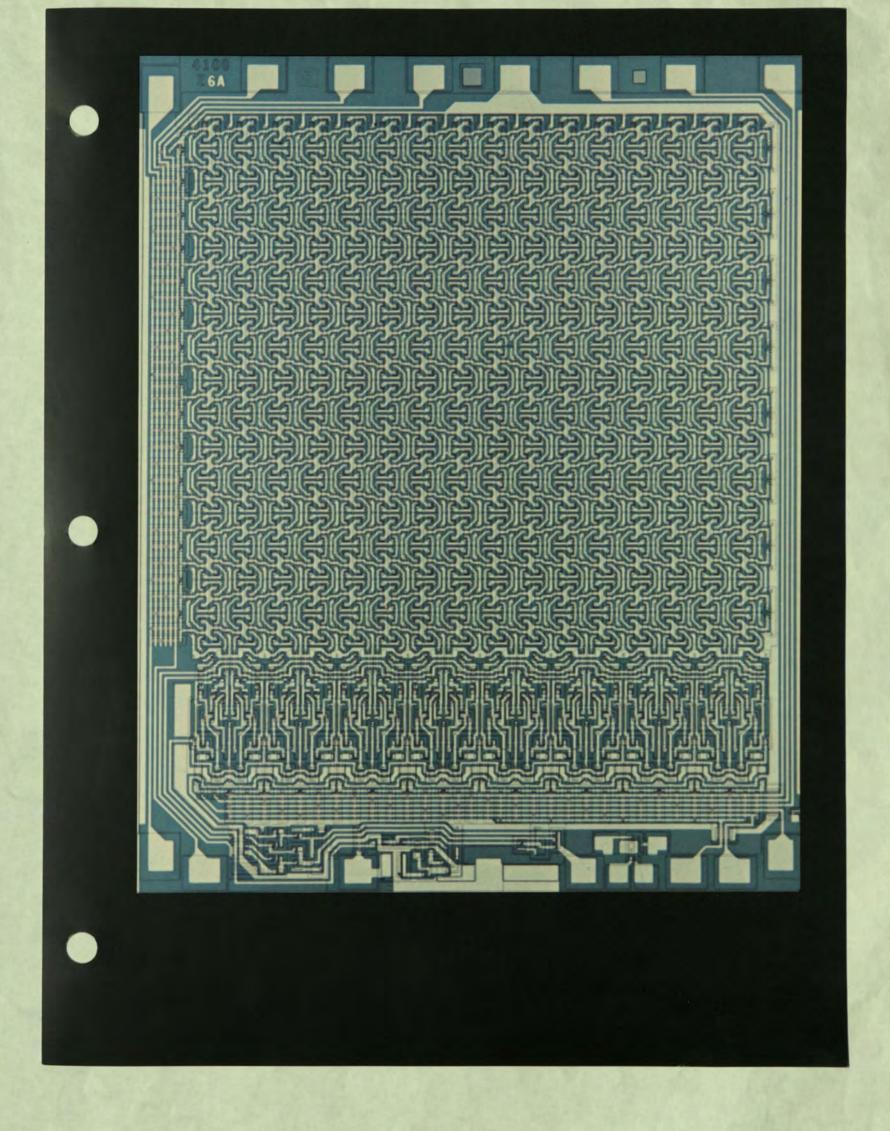
A 128-element linear sensor—Fairchild's first self-scanned photo array.
