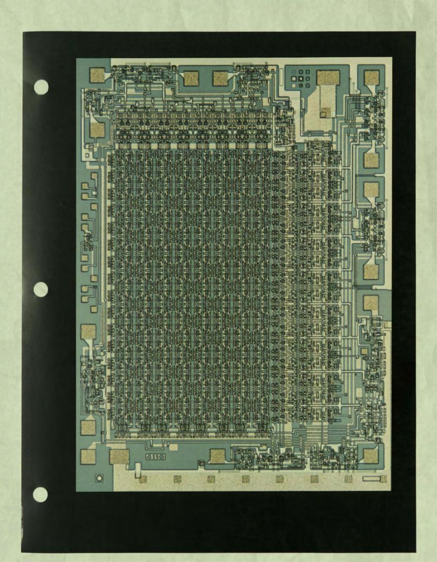
This monolithic voltage regulator was the first such product to be completely self-sufficient on a single silicon chip, with no external components needed for operation.
