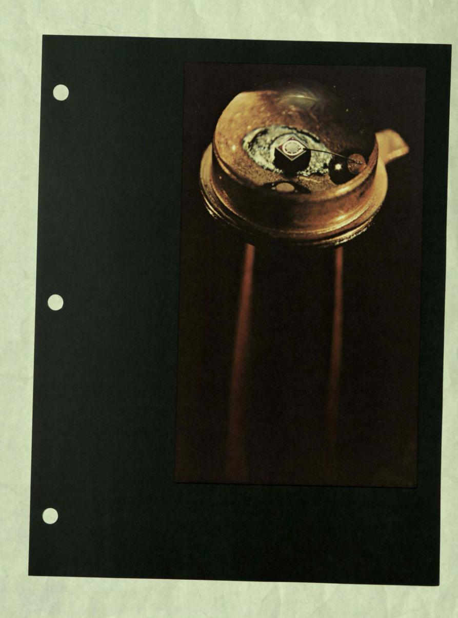
The interconnection masks on this device were generated on Fairchild's computer-aided design system and implemented with the first three layer metal process. This is a 48-gate custom TTL logic array.
