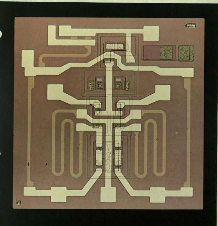
This low-power, high-frequency (700 megahertz) PNP transistor was among the earliest extremely fast epitaxial devices in the industry.
