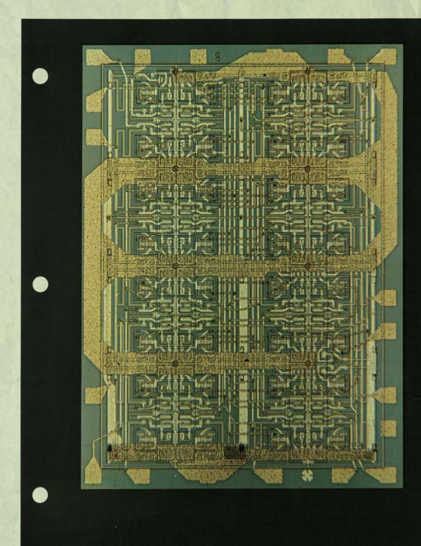
This operational amplifier was one of the earliest linear integrated circuits to include temperature compensation and MOS capacitors.
