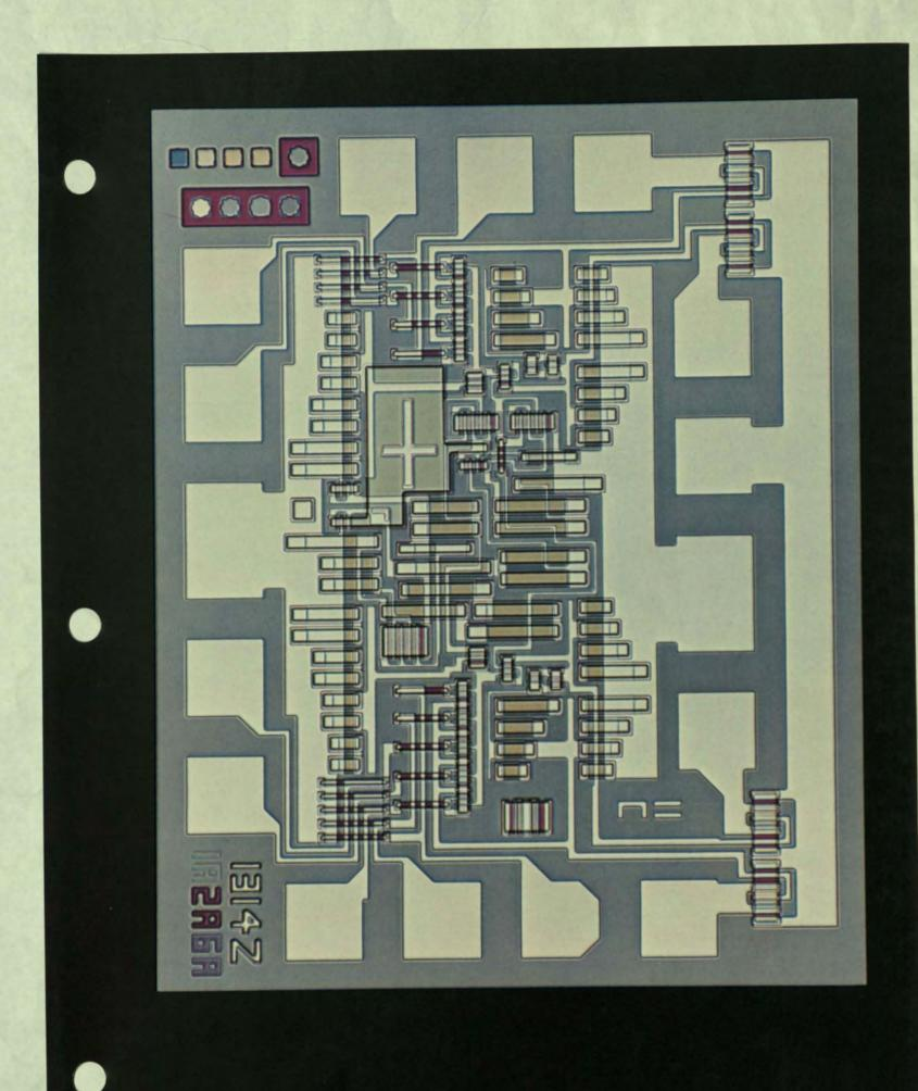
The world's first commercially available charge-coupled device (CCD)—a 1 x 500-element linear image sensor, 636 mils long. The individual elements, which are just 1.2 mils from one another, are also shown in a closeup view. This monolithic N-channel device, under a sealed glass window, includes a 500-element photosensing strip bounded by two 250-element CCD analog shift registers and a two-element CCD output register which transfers charge to an on-chip NMOS buffer device.
