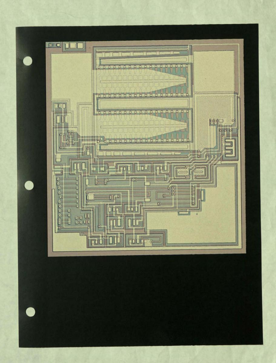
This emitter-coupled logic (ECL) version of the first commercial Isoplanar memory is a 256-bit fully decoded memory with even higher speed operation than the TTL version. ECL is the main logic form being designed into computers for the 1980's.
