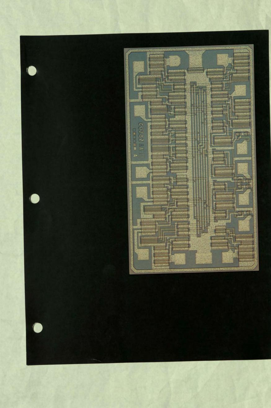
The F8™ microprocessor, Fairchild's first proprietary Isoplanar N-channel product, was the industry's first 8-bit microprocessor aimed specifically at the high-volume, low-cost control market.
