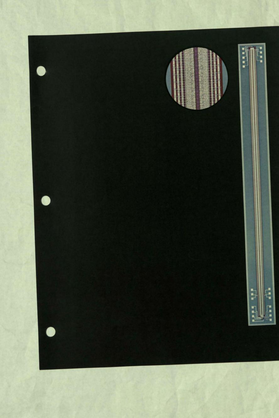
Fairchild's first Isoplanar MOS product. This P-channel device is a 1,024-bit static register. It represents a 30 percent reduction in chip size from previous MOS devices with comparable capability.
