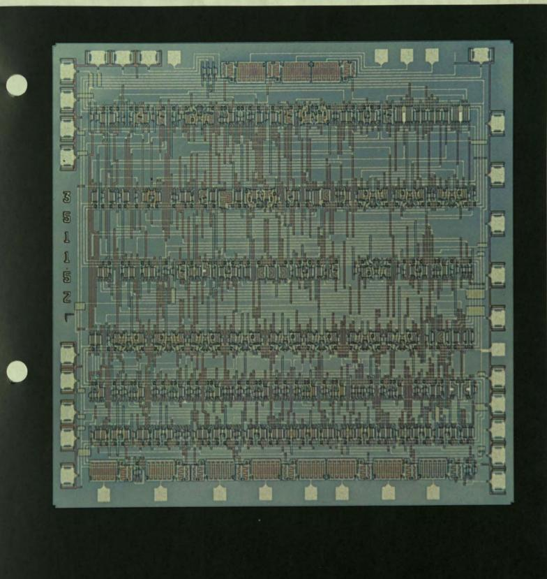
The world's first commercial Isoplanar™ product. A 256-bit fully decoded bipolar random access memory chip. DTL/TTL compatible with a 50-nanosecond access time.
