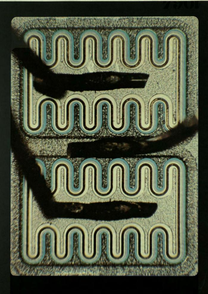
Fairchild's first radio frequency power transistor—a 1-watt, 300-megahertz device.
