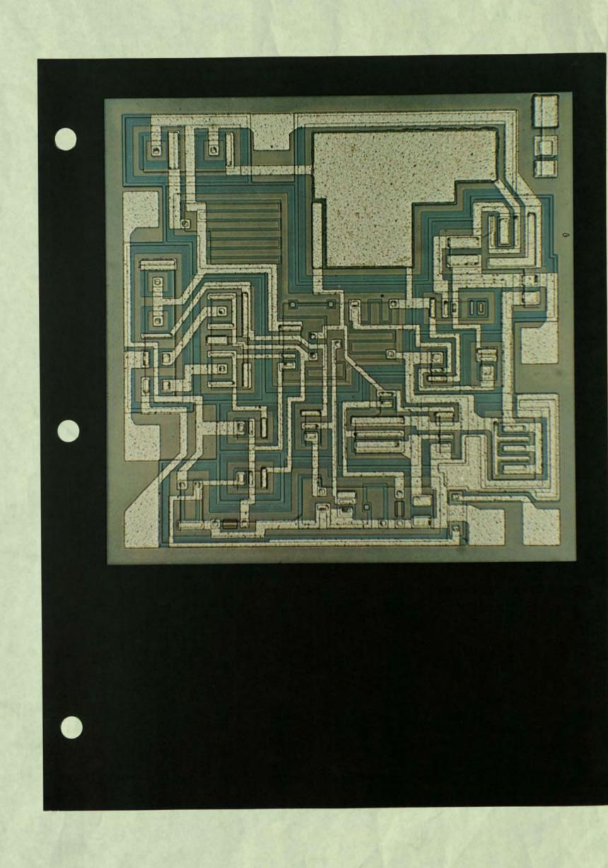
The first silicon gate product with TTL compatible digital input logic. An eight-channel MOS signal multiplexer.
