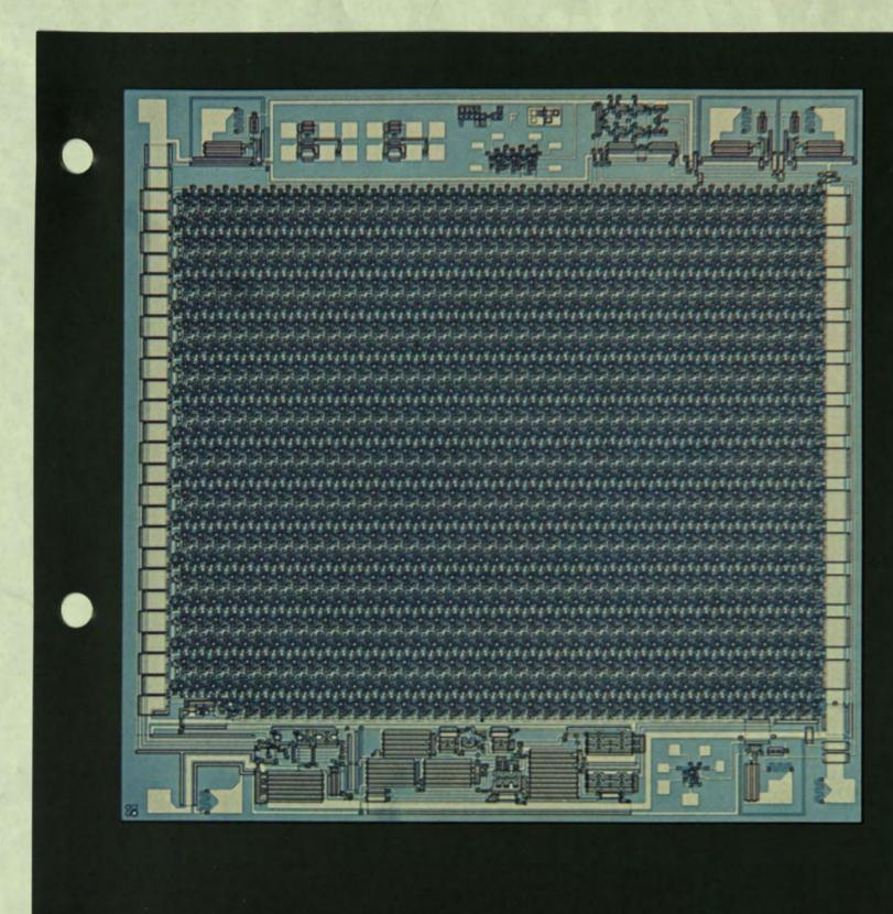
Fairchild combined Isoplanar technology with CMOS (Complementary MOS) structures to provide a widely accepted family of CMOS logic devices with the smallest chip sizes and highest speeds in the industry.
