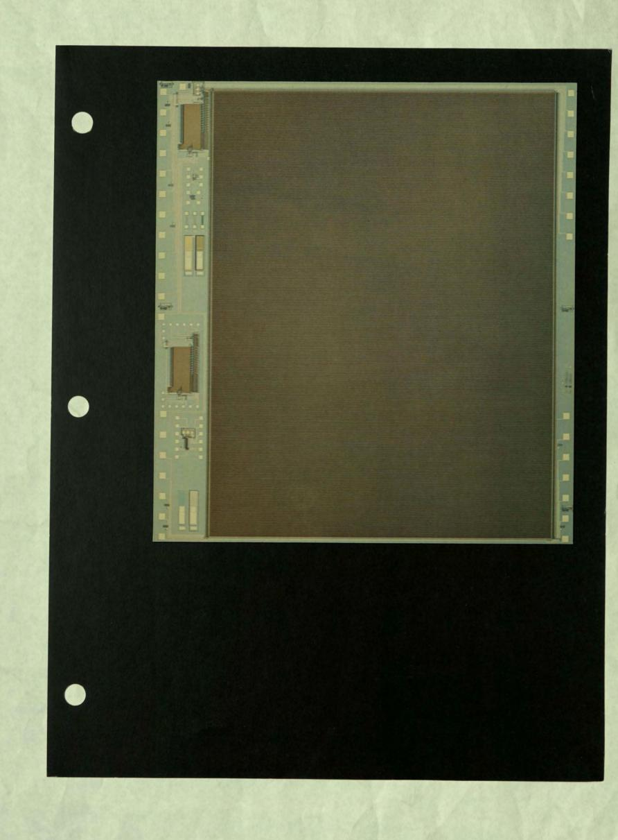
The 9440 16-bit microprocessor is the first integrated circuit with the capability of a minicomputer CPU (Central Processing Unit) on a single chip. Utilizing Isoplanar Integrated Injection Logic (I³L)™ technology, the 9440 operates at true minicomputer speeds of 10 megahertz and above.
