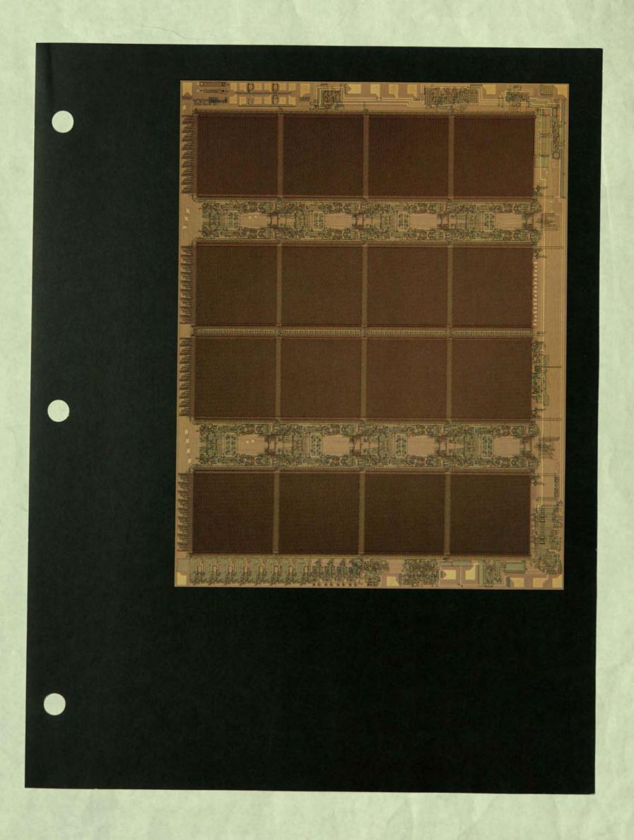
This CCD (Charge-Coupled Device) area image sensor contains an array of 488 x 380 imaging elements on a single chip of silicon. Approaching 300,000 elements, this device easily represents the highest number of circuit components on a production chip. The sensor provides the highest resolution of any currently available silicon imaging device.
