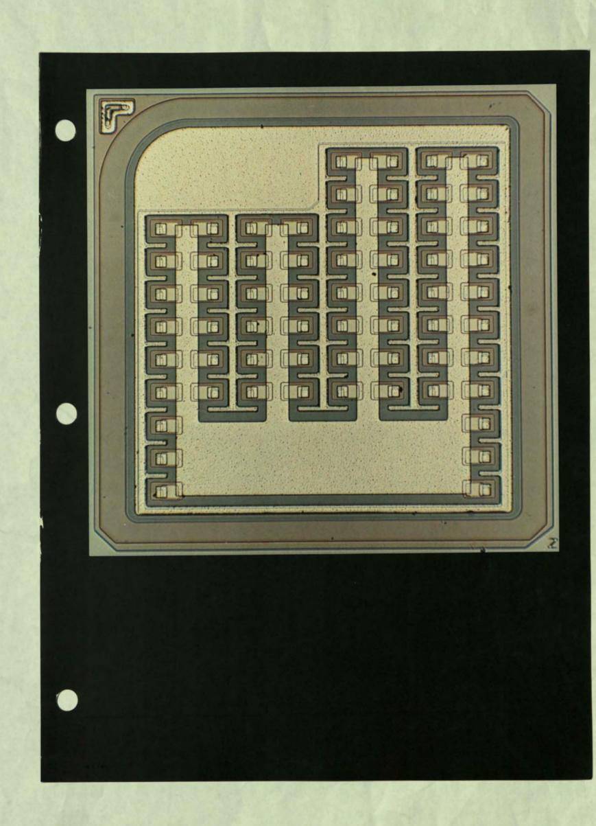
The first custom large-scale-integration (LSI) device evolving from Micromosaic techniques in a computer-aided design system. This is a 150-gate MOS random logic device.
