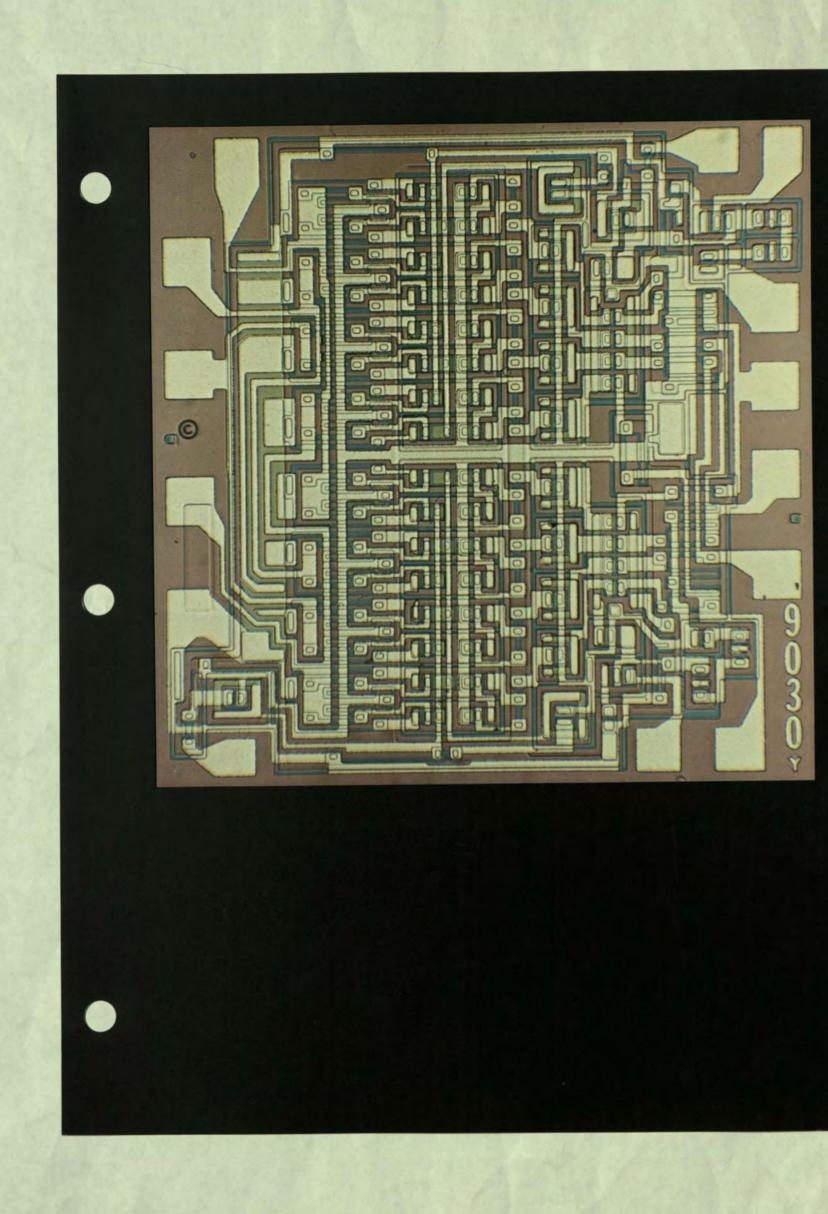
The first monolithic 10-bit current source for digital-to-analog converters. A unique  $157 \times 60$  mil size.
