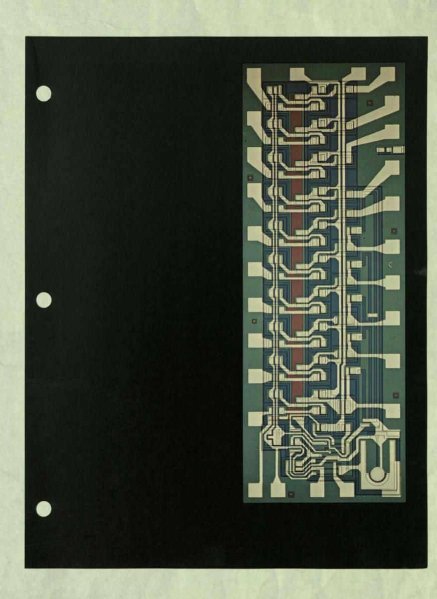
The industry's first two-layer metal process put into production. A 32-gate custom DTL logic array.
