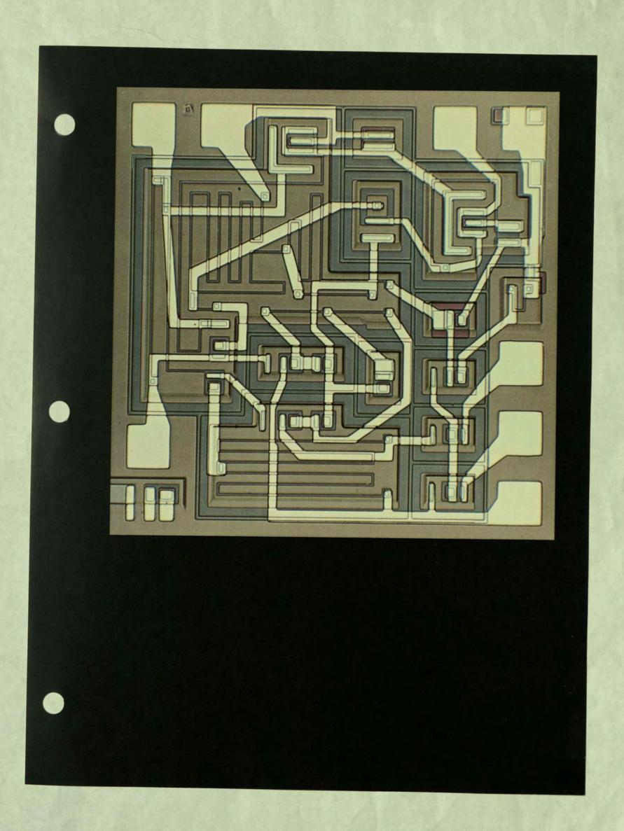
This DTL triple-gate device was the first radiation hardened product made with dielectric isolation and thin-film resistors.
