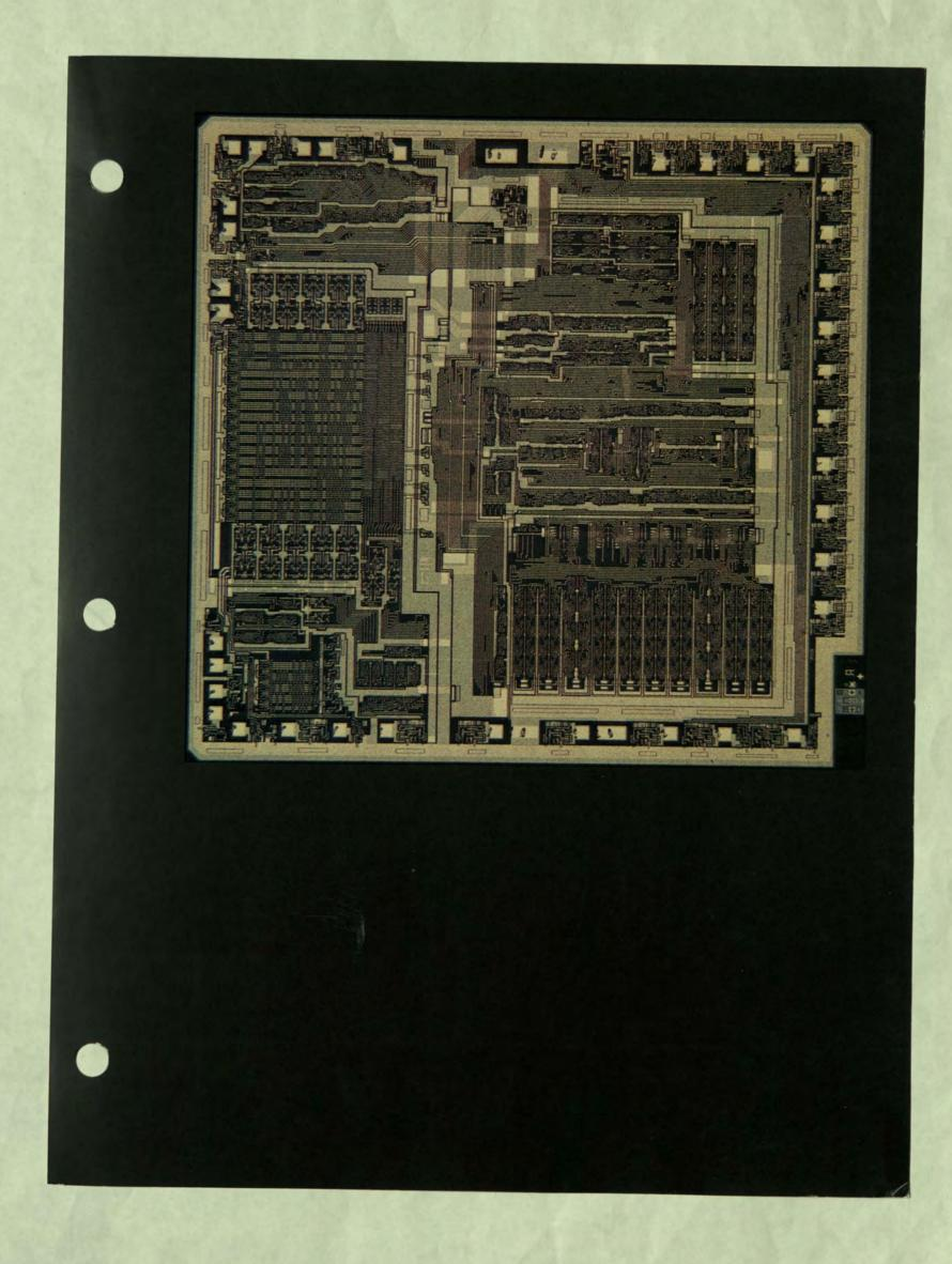
This 16,384-bit Isoplanar Integrated Injection Logic (I³L)™ dynamic RAM (Random Access Memory) further advances the performance of MOS circuitry with operating speed approaching that of bipolar devices.
