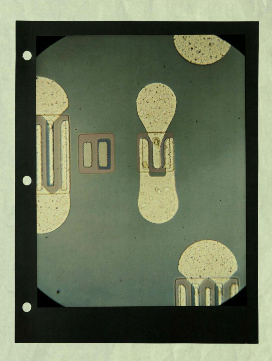
The dawn of the integrated circuit era. This resistor-transistor logic (RTL) product—a set/reset flip-flop—was the industry's first integrated circuit available as a monolithic chip.
