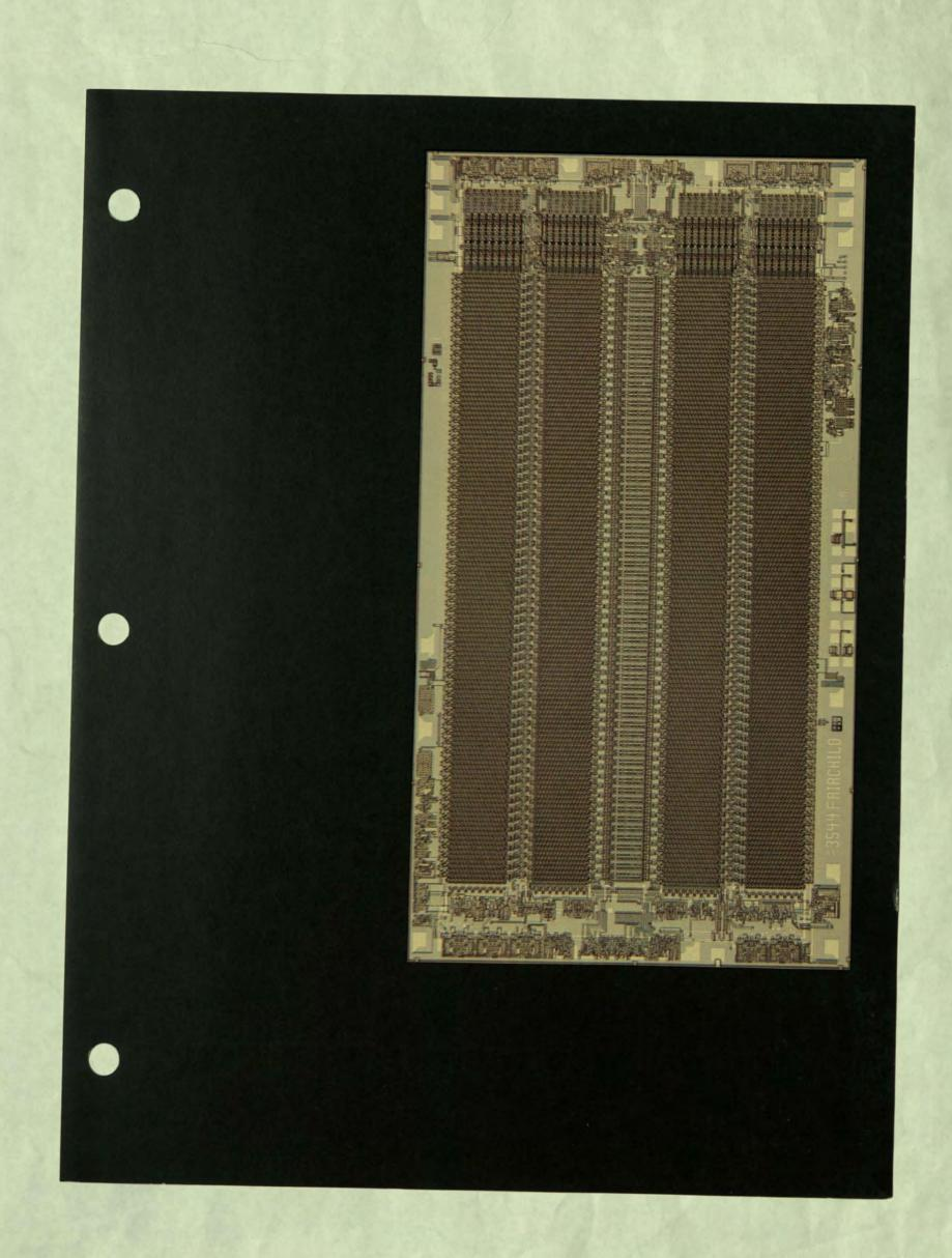
The 65,536-bit CCD (Charge-Coupled Device) memory is the most complex integrated circuit memory. It combines all currently available advanced MOS circuit techniques, including double-layer polysilicon, ion implantation and Isoplanar structures. This is the first semiconductor memory capable of being cost competitive with bulk storage devices such as fixed-head disk memories.
