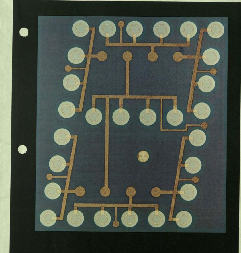
The first solid-state random access memory in production. This 256-bit partially decoded bipolar memory was used in the Illiac IV computer.
