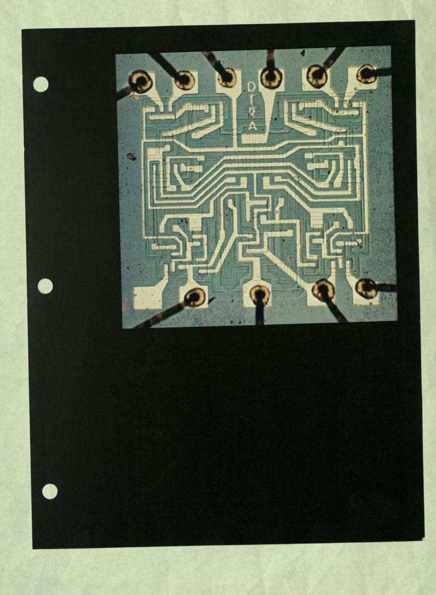
This dual-gate, custom transistor-transistor logic (TTL) design was used in the first commercial application of TTL logic.
