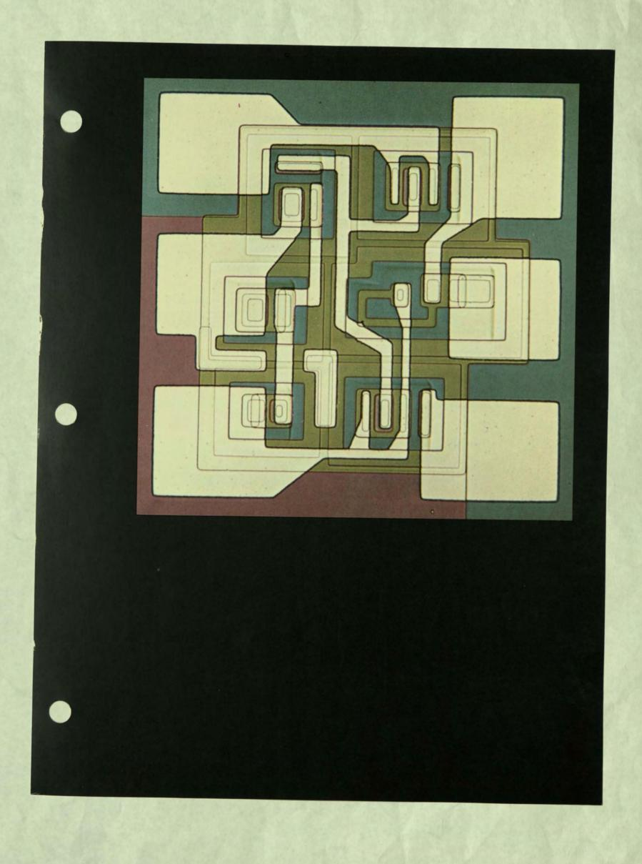
A milestone in the linear integrated circuit field, this device—the  $\mu A709$ —was the first operational amplifier generally used throughout the industry.
