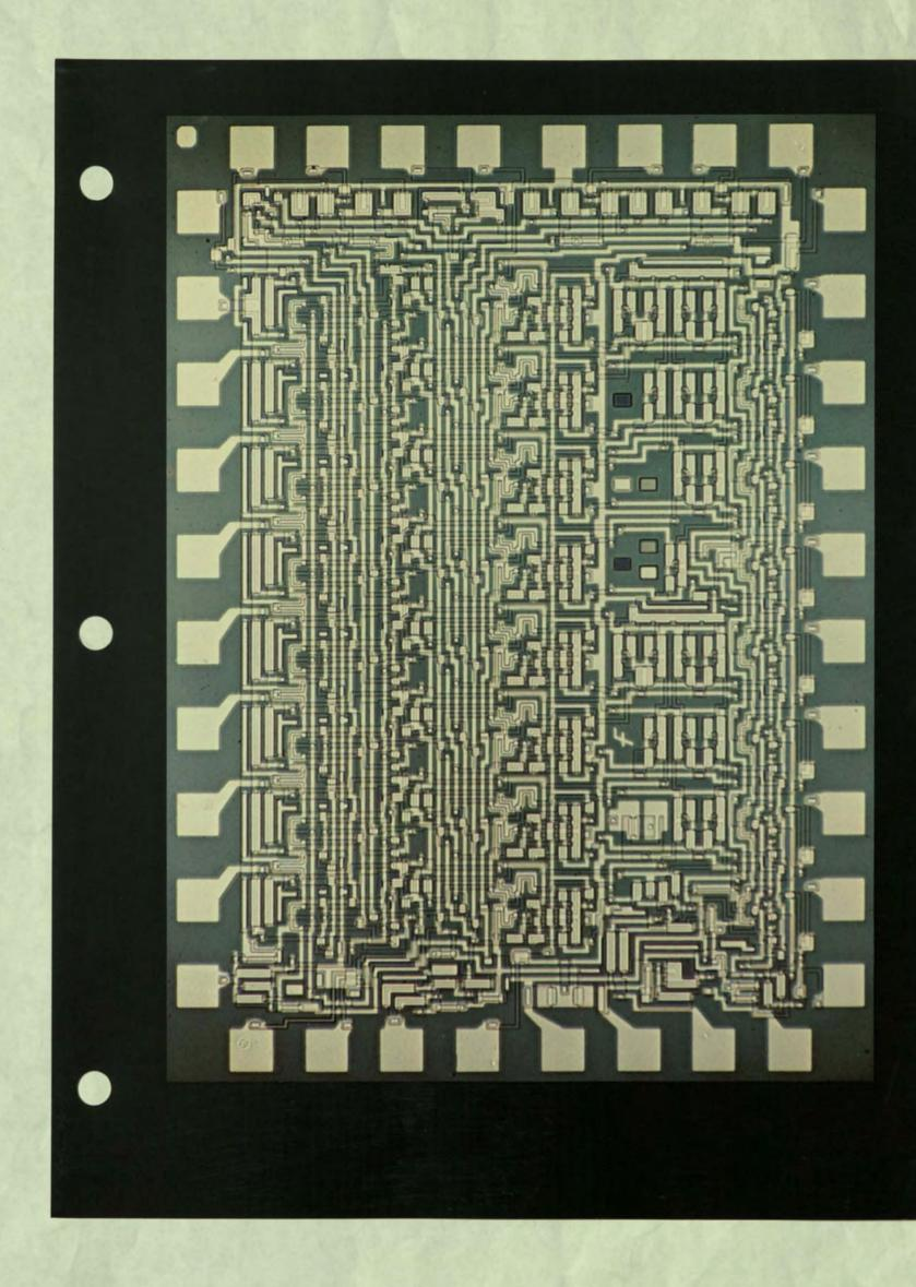
The first complementary-transistor logic (CTL) medium-scale-integration design—an eight-bit latch for high-speed register applications.
