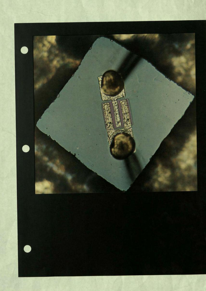
A second generation RTL product, this dualgate device was the first to incorporate buried-layer isolation technology.
