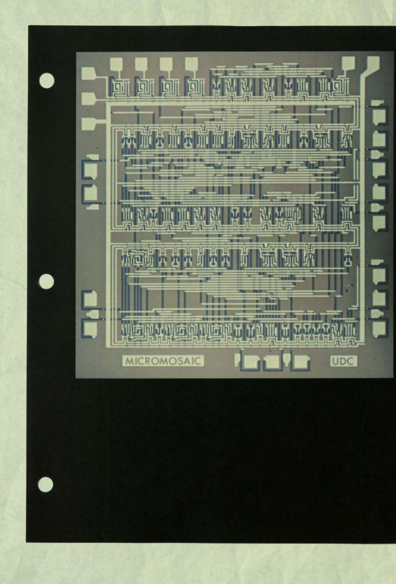
The first standard MOS product for data processing applications—an eight-bit arithmetic unit and accumulator.
