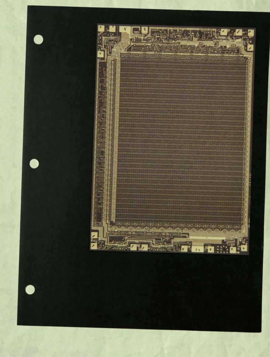
Fairchild's 16,384-bit N-channel dynamic RAM (Random Access Memory) utilizes Isoplanar processing to achieve the smallest chip size and highest speed of any 16K MOS RAM. In addition to high performance, the small size of this device allowed the use of a standard 16-pin package, an important cost reducing feature.
