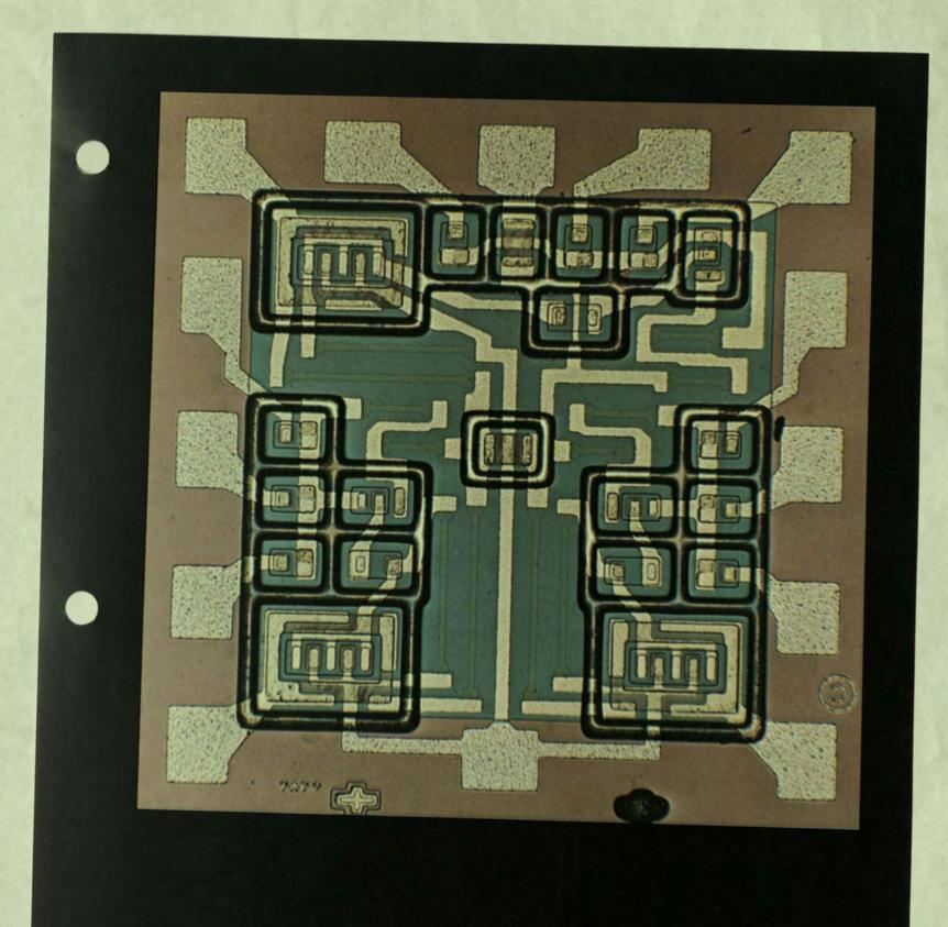
The industry's first gold-doped PNP transistor, made with a stabilization technique that utilizes an equipotential ring.
