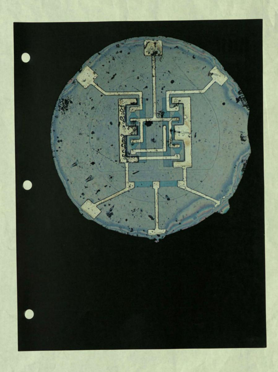
A standard product that served as the industry's workhorse for discrete logic—the first widely accepted epitaxial gold-doped NPN transistor.
