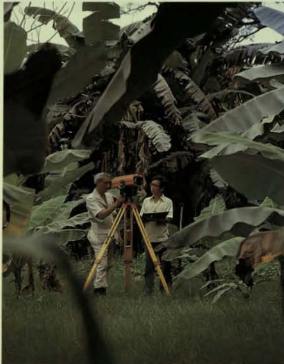
HP's total station distance- and angle-measuring instruments made land surveying faster and easier, such as this scene of an Australian engineering crew in Kuala Lumpur, Malaysia.
