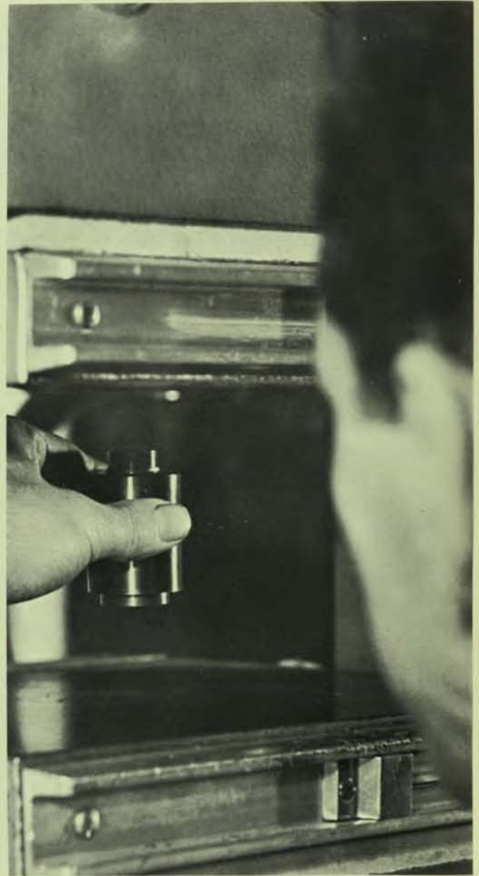
Converting non-conductive plastic into conductive function elements for precision potentiometers requires special equipment and techniques perfected by Fairchild Controls. Here a technician is placing a capsule containing a "raw" element into heat press where conductive "track" will be integrally co-molded into the non-conductive base.
