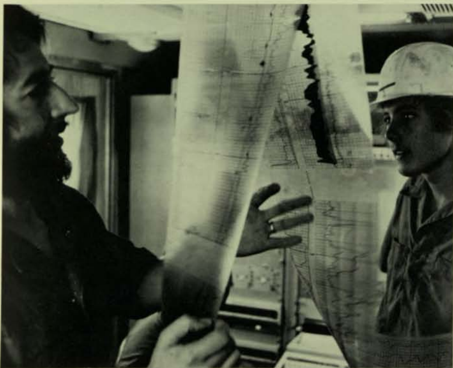
Above, a drilling operation off Indonesia. Far left, engineers check for abnormal pressure trends on a Measurement While Drilling (MWD) log running in real time during Gulf of Mexico drilling. Left, a log printout provides vital information to field engineers in Saudi Arabia.
