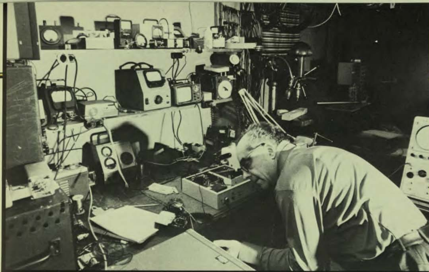
Much of Ed's spare time is spent in his basement workshop, constructing and testing ATV equipment. Experimental repeaters take the weak signals sent out by home transmitters and rebroadcast them on a slightly lower and stronger frequency. Once the Long Island system is fully operational, Ed says the picture transmitted will be as sharp and clear as a commercial television broadcast.
