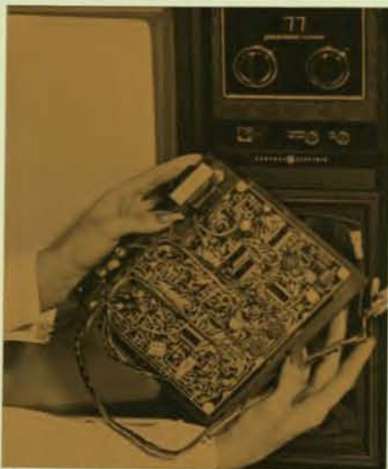
This single modular circuit board decodes the VIR signal and automatically adjusts the picture.
