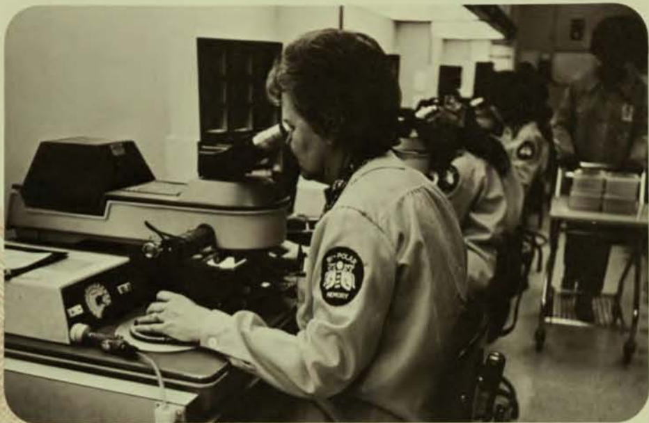
A Bipolar operator aligns glass photomask over a silicon wafer during fabrication of Isoplanar memory circuits. Ultraviolet light exposes the wafer to the pattern of circuit elements on the photomask.
