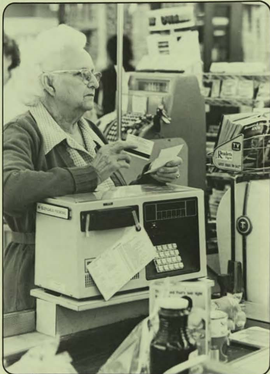
Elsie Williams, Glendale Federal Savings customer, waits with identification card in hand to electronically charge groceries to her Glendale account. While a checker scans her card and records the transaction, Elsie will punch a secret code number on the EFT terminal.
