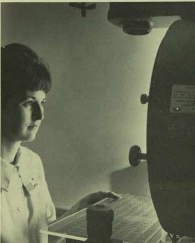
Carole Chrisman needs a sharp eye to measure frames on the Comparator. The frames must conform to specifications shown on the screen.
