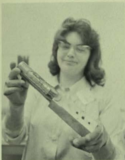
6. After flattening, the ingot is fastened to a metal bilet with heavy wax. Norma Moreno holds a mounted crystal, ready for slicing into wafers.
