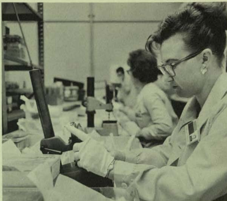
9. Ruth Whitley and her co-workers then classify the wafers into 5\mu groupings. Each wafer is given a diameter check and type test (for resistivity).
