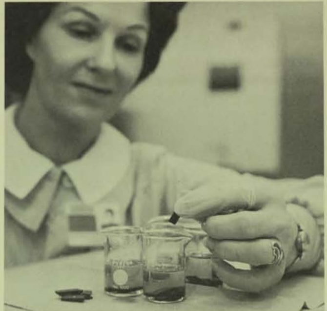
Kitty Troncoso submerges Dip bases in a chemical solution, Zygo. Each beaker is placed in a pressurized "joy bomb" to check the porosity of the ceramics.
