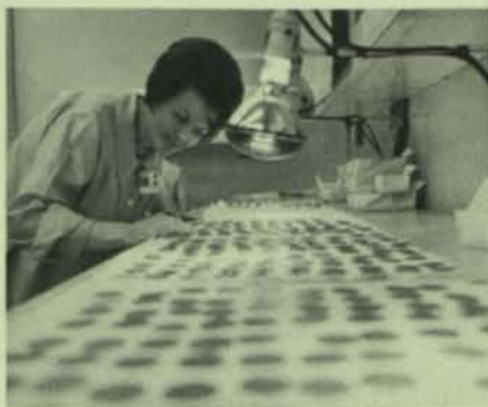
8. The wafers are carefully removed from the bilet, washed, and dried under an infrared light. Betty Childers gazes over a sea of slices that are drying.
