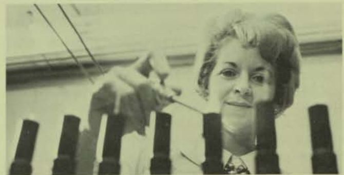
The sample is categorized and checked according to military specifications. Running the Glass Seal Test on TO-18 Nail Headers, Dee McGowan uses helium to check for leakage.
