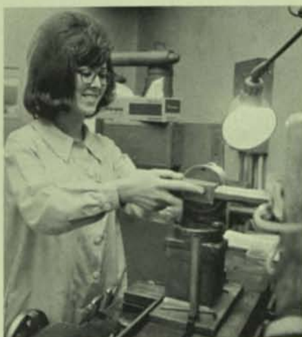
7. Delrene Vazquez inserts the metal bilet into the arm of an automatic slicer. A diamond blade cuts the crystal into wafers, 10 mils \pm .5 mils in thickness. One silicon ingot produces an average of 140 slices.
