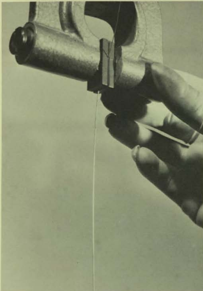
The breaking strength of gold and aluminum wires is checked as is its elongation.
