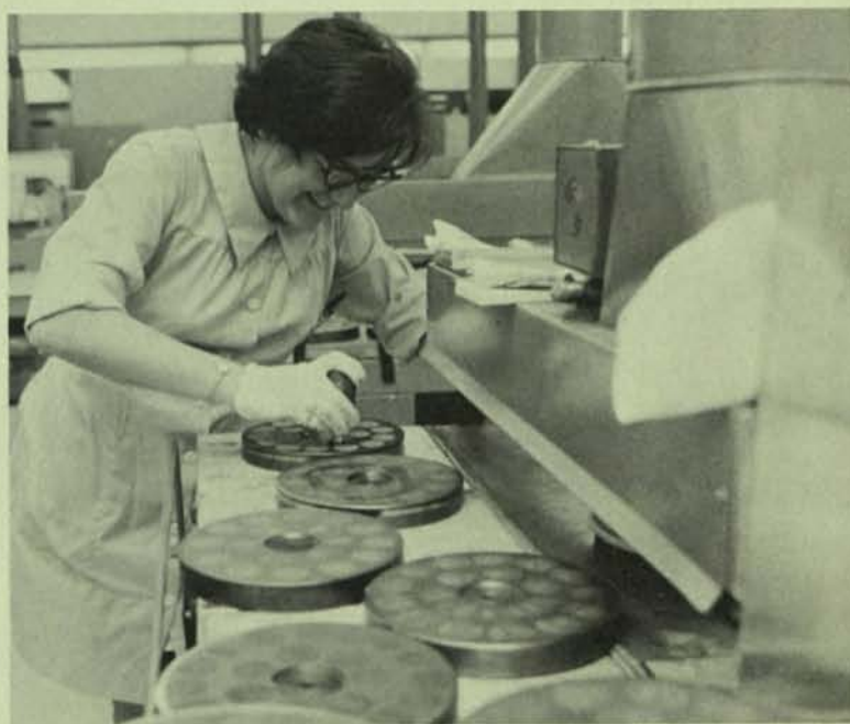
10. Following evaluation, wafers go either to Lapping or to Polishing. In each case, however, they must be waxed down on grinding discs before further processing. Diane Bailey adheres wafers to discs which have been warmed on hot plates and coated with wax.
