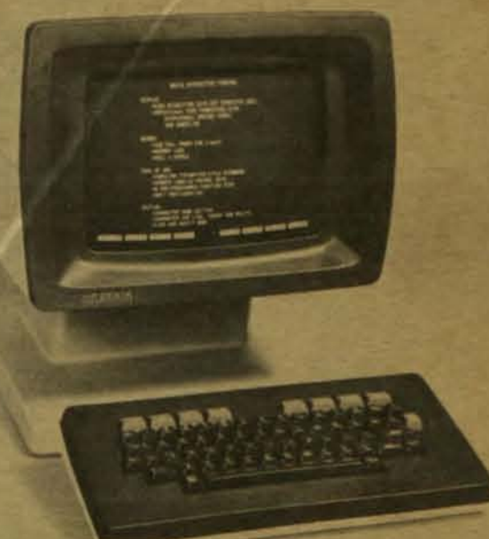
The Hewlett-Packard 2621A CRT terminal, the lowest priced HP CRT available, offers the user a high resolution screen and 4k bytes of memory.
