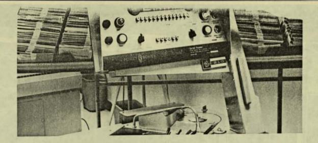
The Document Sorter/Readers, earlier described as the "eyes" and "hands" of the ERMA system, are capable of being operated in two ways. These are known as "on-line" or "off-line."
