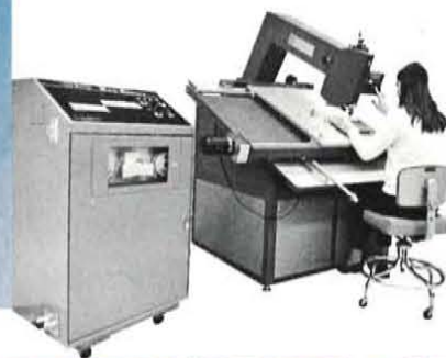
Automatic wire wrapping of central processing unit
