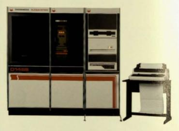
The D148S is the output portion of the DICOMEDIA SLIDESYSTEM, accepting input from DICOMED's D38 Design Station or other compatible graphics systems to create:
