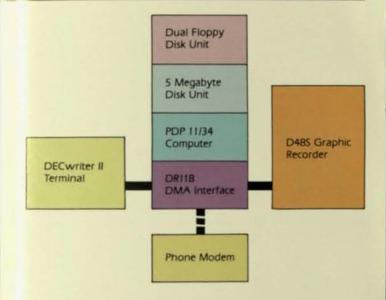
Through its UNIBUS system architecture, the PDP 11 control computer provides a highly flexible means of system expansion. System components such as graphic displays, printers, and additional film recorders may be readily added to the System. The magnetic tape controller and the disk subsystem provide for the easy addition of magnetic tape transports and disk drives, respectively.
