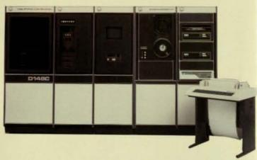
The DICOMED D148C Color Graphic COM System is a standalone computer-output-to-microfilm system with outstanding color graphics performance. It provides a unique optical system to produce high-fidelity color in a continuous spectrum.
