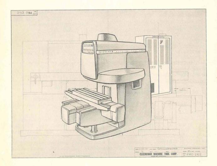
The Spindlemaster is a new concept in <u>low cost</u> "flexible automation." This tape controlled machine, a Manufacturing Engineering Service development, should find wide application in the General Electric Company. The project was undertaken by Advanced Manufacturing Engineering Service in an effort to create new sources for advanced equipment designs that would most effectively meet the needs of General Electric Operating Departments.
