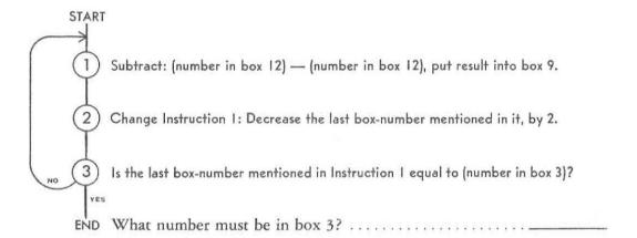
The purpose of the following flow-chart is to add the numbers in boxes 7, 8, 9, and 10 and put the total into box 2.
