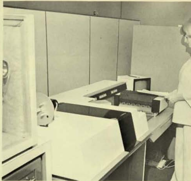
Composing department staff member at the Daily Times-Advocate (Escondido, Calif.) shown putting copy in stack feeder of Compu-Scan optical character scanner. Punch for paper tape output is at left.
