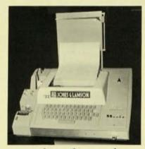
tape and simultaneously deliver a complete program read-out, at the press of a button! What's more, in many cases you can dry cycle the machine tool directly from the Editor to prove the program *before* punching the tape.
