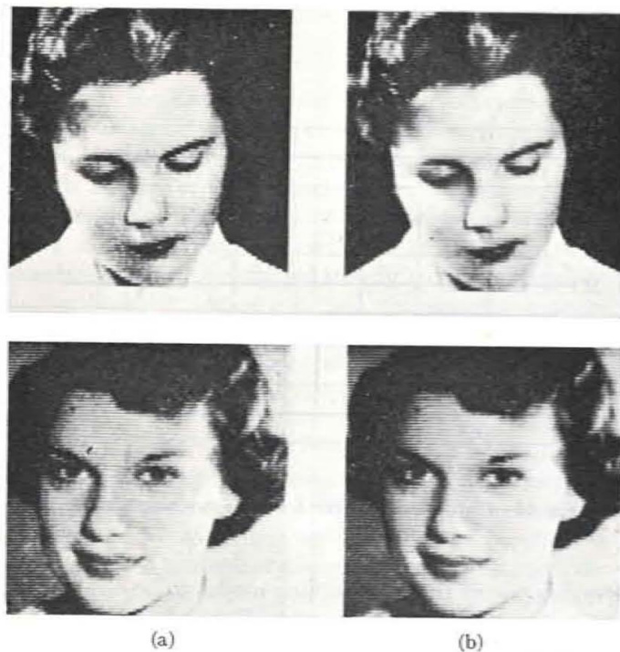
Fig. 11—Typical results from simulation of noise stripping operation. (a) Unprocessed. (b) Processed.
