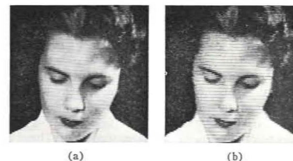
Fig. 8—Comparison of picture codings. (a) 3-bits/picture point, differential quantizing. (b) 3-bits/picture point, pulse-code modulation.
