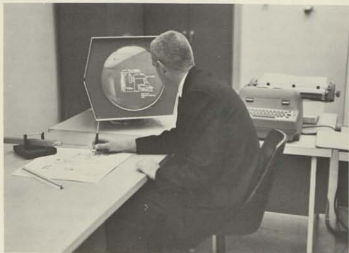
2. Light pen modification of a computer-displayed graph which has been generated by sorting of hospital movement data. 2
